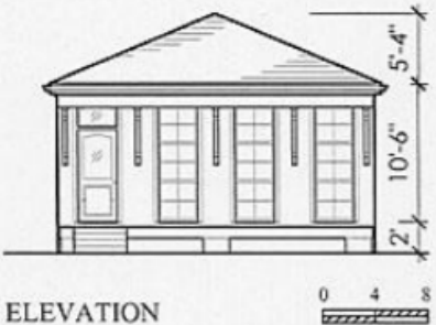
62 | Examples of a standard, traditional four bay single barrel (right) and double barrel shotgun house (left) in plan and elevation
