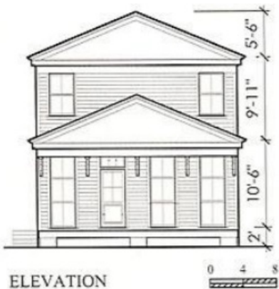
61 | Example of a standard, traditional four-bay single barrel, camelback shotgun house in plan and elevation
