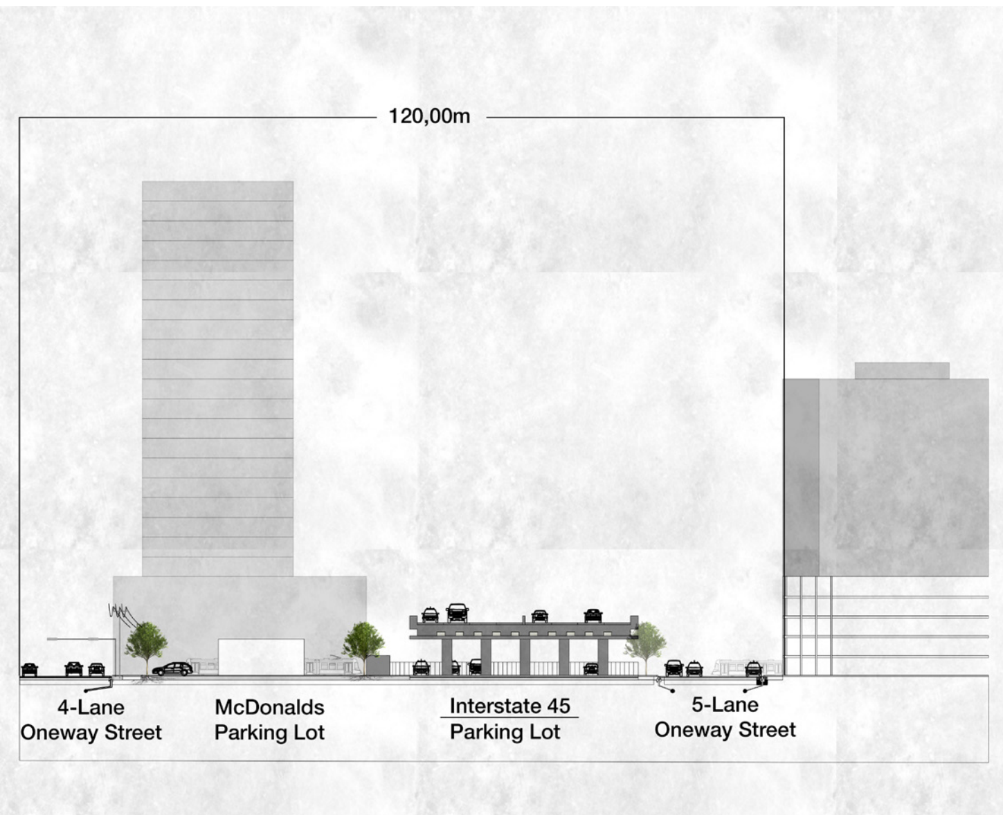
BEFORE: A section of the I45 between Downtown and Midtown showing the space dedicated to cars on different layers. The unwalkable and unattractive area creates a barrier between different neighbourhoods. A high level of impervious surface increases run-off and intensifies the risk of flooding.
