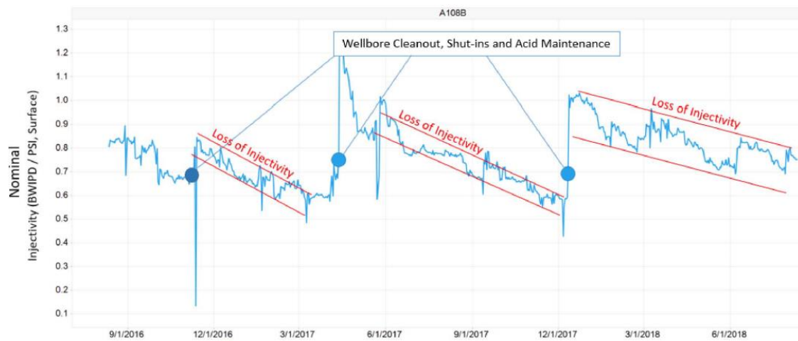
Figure 1.3: Wilmington field (California) performance, where loss of injectivity is demonstrated [13].
