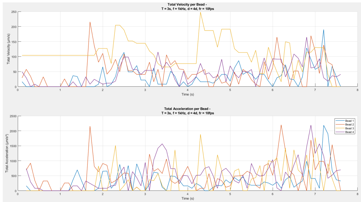
Figure D.1: The measured velocities and accelerations of the 15 \mu\text{m} polystyrene beads in the OET with a medium of deionized water with 0.05% Tween-20. The used sweep animation had a sweep time of 3 seconds and a thickness of 120 pixels. The voltage on the chip was 30 V with a frequency of 1 kHz.
