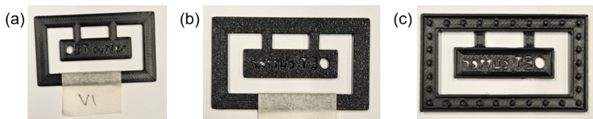
Figure 3.14: The 3D printed channel cutters. (a) shows the front side of version 1. (b) shows the back side of version 1. (c) shows the back side of version 2.
