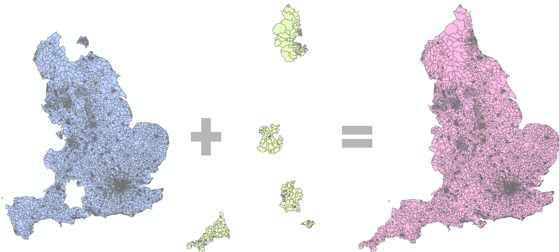
Fig. 33: Joining of the two layers with administrative units the 5th level in the administrative hierarchy
