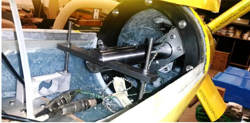
**Figure 4-5:** Inner end of the shaft and its connection to the force sensors for the total torque measurements. One of the sensors can be seen on the left.
