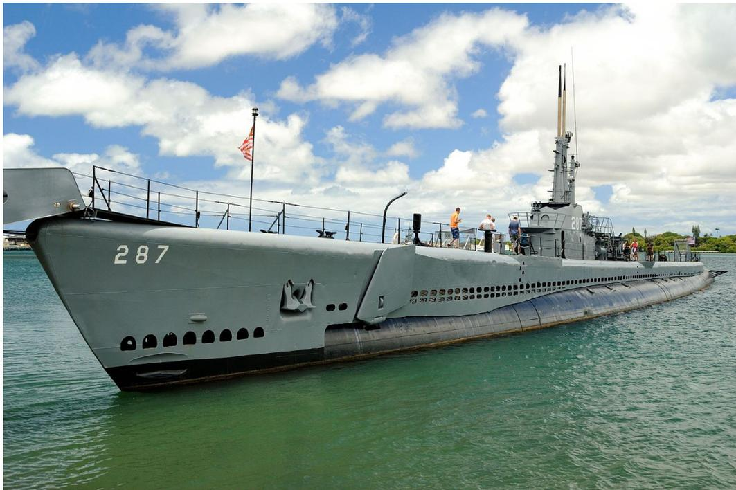
**Figure B-1:** USS Bowfin, a submarine from the second world war era, showing the casing in light grey on top of the pressure hull in dark grey. Interesting is also the folded bowplane just aft of the anchor.
