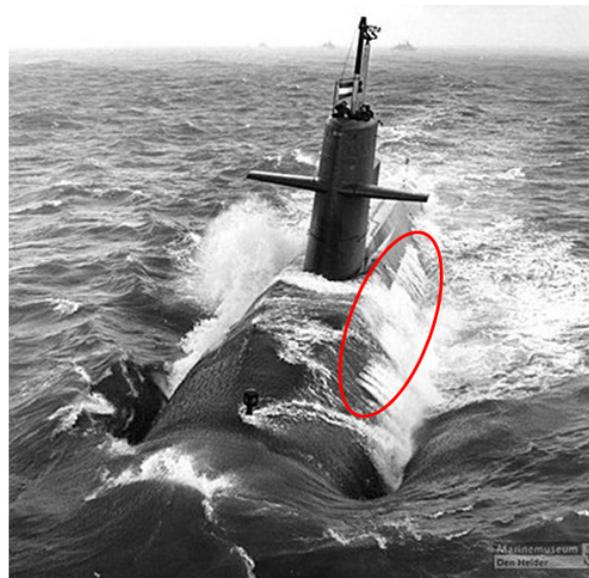
**Figure B-2:** Flood gates of a surfaced submarine. Water can be seen to escape through the port flood gates (inside the red ellipsis).
