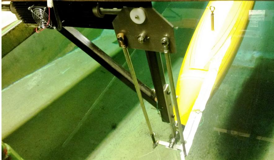
**Figure 4-4:** The linear motor, with the two connecting rods and the aft part of the shaft that transfers the roll motion to the model.
