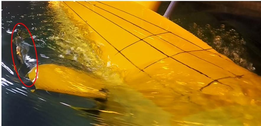
**Figure 3-3:** The tip vortex from the starboard bowplane is visible as a depression in the water surface behind the bowplane, within the red ellipse.
