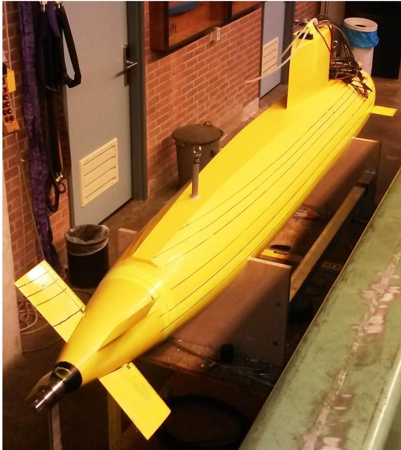
**Figure 4-1:** The model used in the experiments, with large X-rudders and bowplanes mounted.
