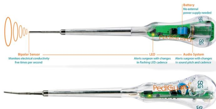
FIGURE 2.19: Electrical conductivity measurement device for open procedures. Figure from [50]
