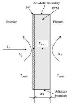
**Figure 2.6:** Schematic diagram of the heat transfer in a PV/PCM system [38]
