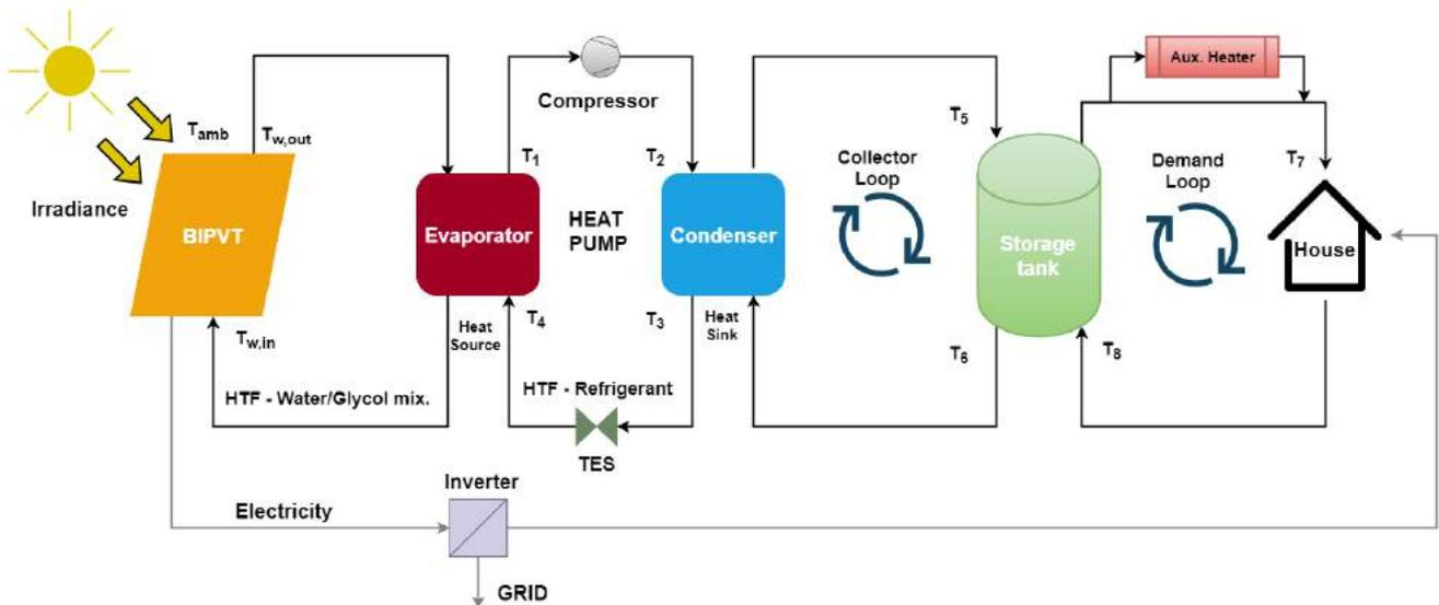
Figure 4.13: BIPVT/Heat pump System Overview
