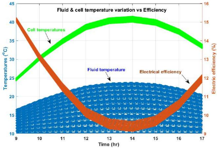
Figure 7.22: Fluid & cell temperature variations throughout the day, against electrical efficiency
