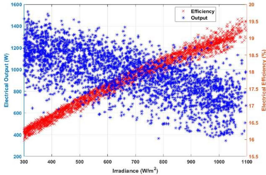
**Figure 7.2:** Effect of irradiance on electrical output & panel efficiency
