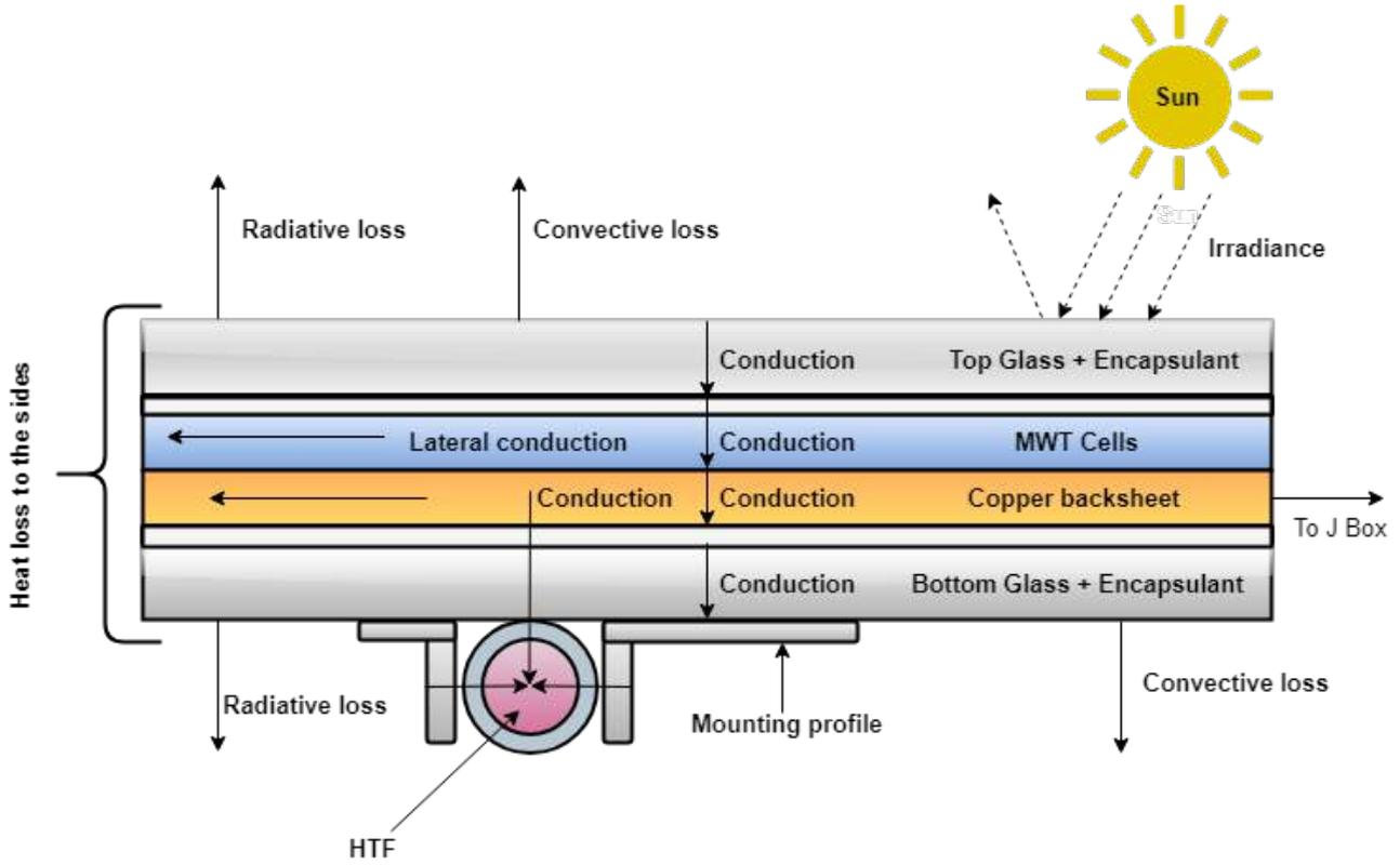
Figure 5.1: Heat flow diagram of the uncovered solar collector
