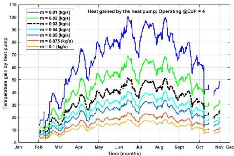
**Figure 7.17:** Heat gained by the heat pump at varying flow rates, operating at  $COP = 4$
