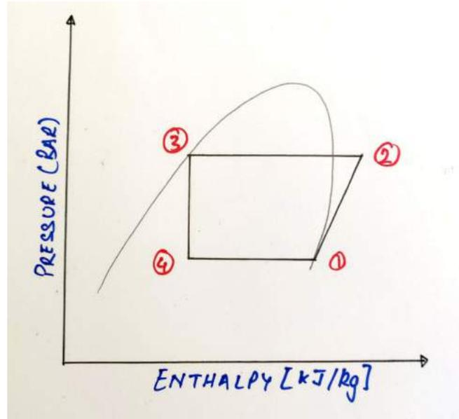
Figure 2.9: Thermodynamic cycle for an ideal Heat pump
