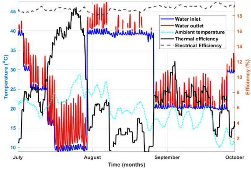
**Figure 7.7:** Water temperature against thermal efficiency
