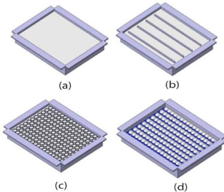
**Figure 2.7:** PCM Configurations - Case a: Bulk; Case b: Finned; Case c: Honeycomb; Case d: Encapsulated [53]
