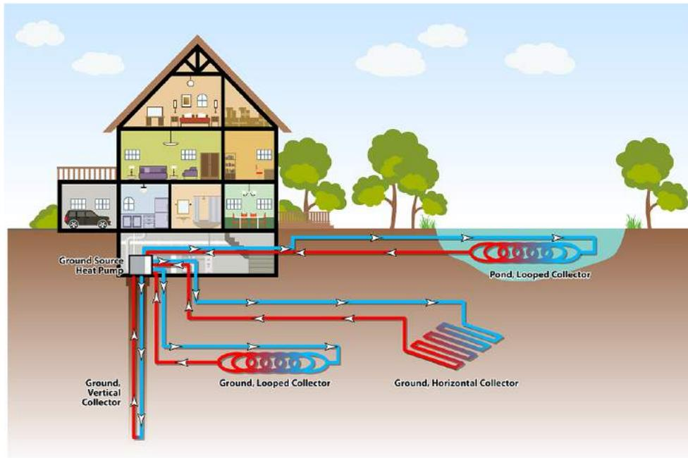
**Figure 2.10:** Geothermal heat pump configurations [13]
