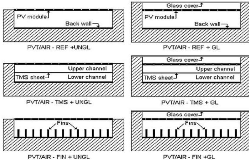
Figure 2.2: Various Air Based PVT Configurations [55]
