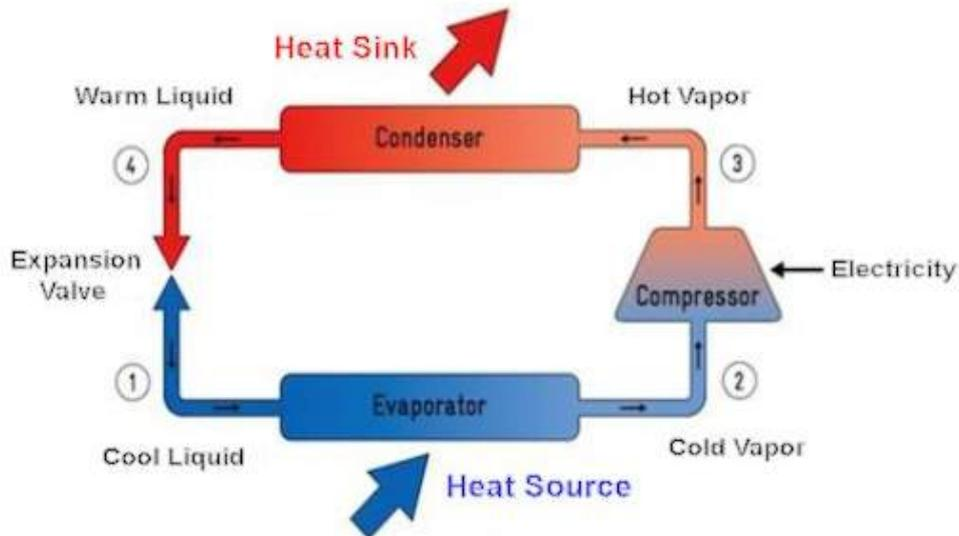
**Figure 2.8:** Heat pump working. A machine that "moves" heat. [Energy]
