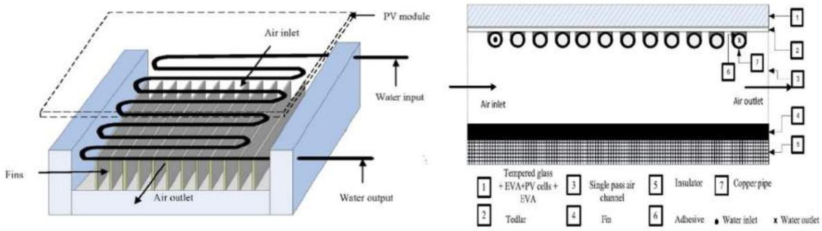
**Figure 2.4:** Bifluid Based PVT System studied by Jarimi et al. [43]
