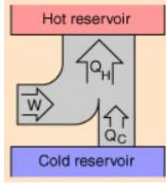
**Figure 5.5:** Heat flow within a Heat pump [3]
