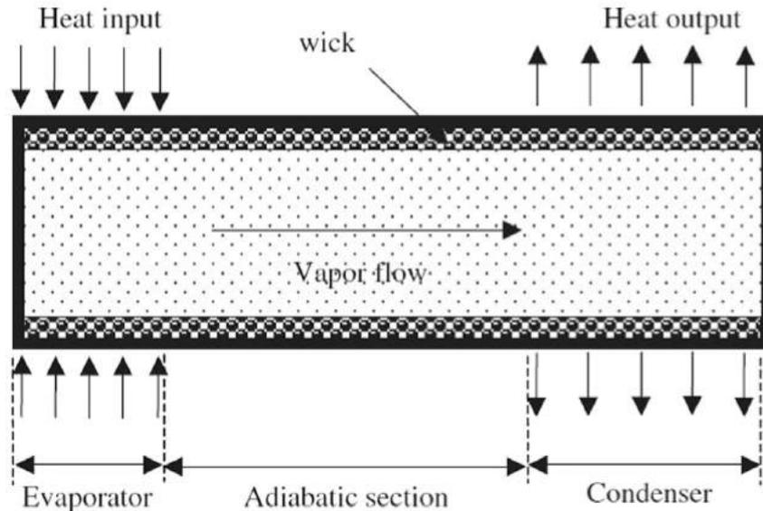
Figure 2.5: Heat pipe schematic [47]
