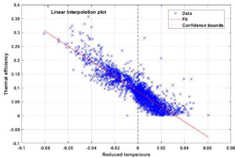
**Figure F.1:** Linear curve interpolation for Steady-state & Quasi-dynamic thermal models
