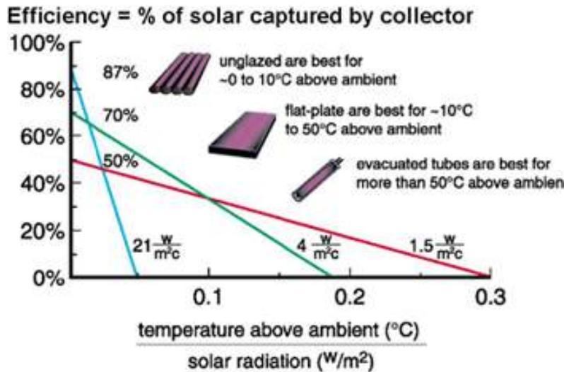
**Figure 5.2:** Typical thermal efficiency curves for unglazed, flat-plate and evacuated tube solar thermal collectors [59]
