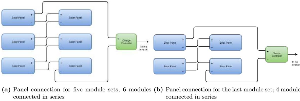
**Figure 4.3:** Experimental Setup panel connections
