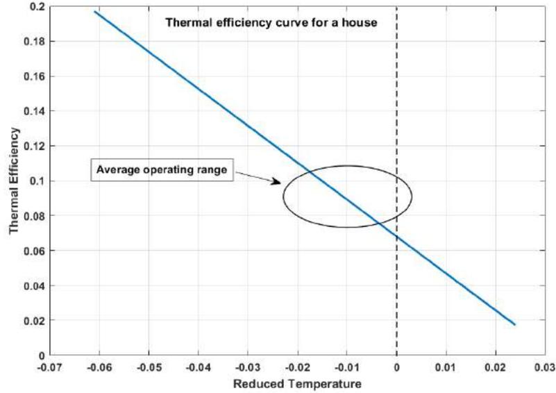
Figure 7.11: Thermal efficiency curve for a house
