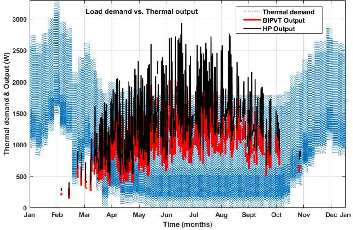
**Figure 7.13:** Load demand vs. Thermal output for the BIPVT & Heat pump
