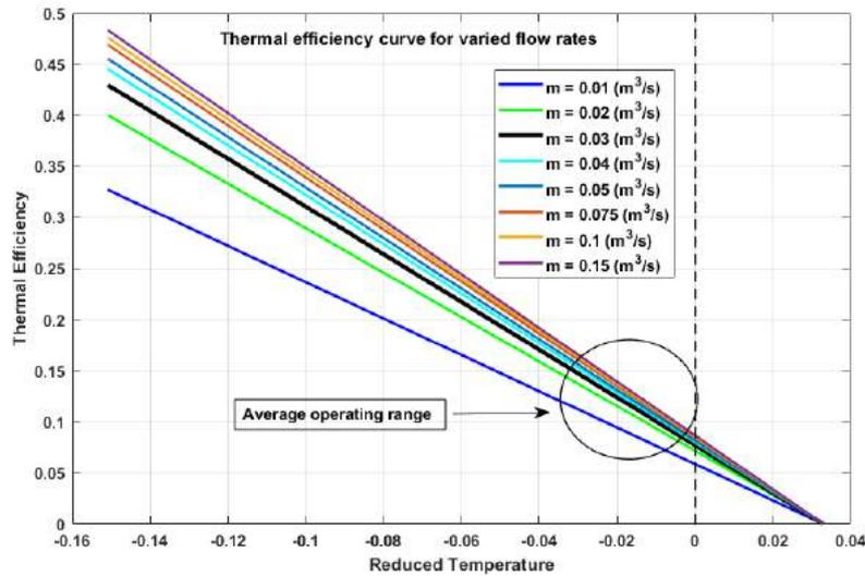
**Figure 7.15:** Characteristic thermal curve for varying flow rates
