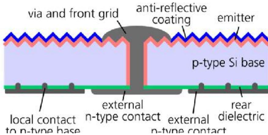
Figure 3.3: MWT-PERC cell side cross-section [12]
