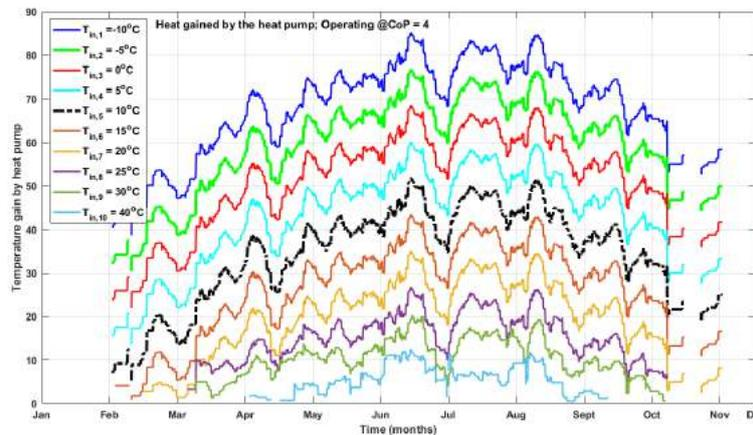
**Figure 7.20:** Heat gained by the heat pump at varying water inlet temperatures, operating at  $\text{COP} = 4$
