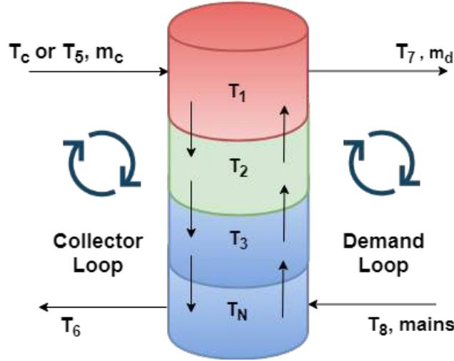
**Figure 5.6:** Overview of a stratified thermal tank
