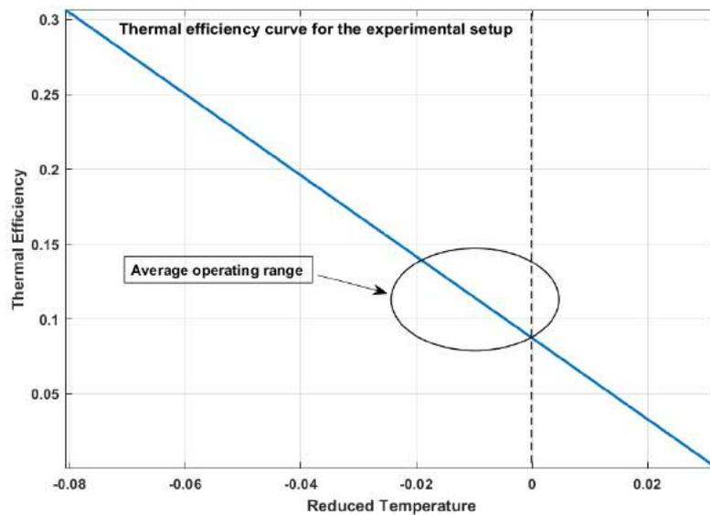
**Figure 7.6:** Thermal efficiency curve for the experimental setup
