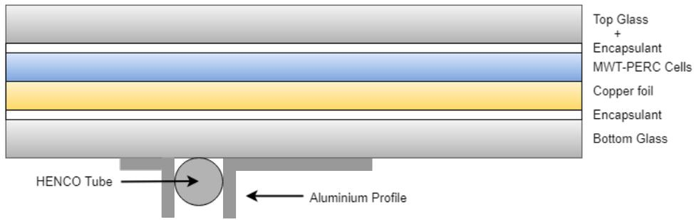
**Figure 3.4:** MWT Solar Panel cross-section
