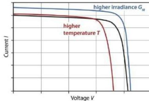
**Figure 7.1:** Effect of temperature on PV Module performance [42]
