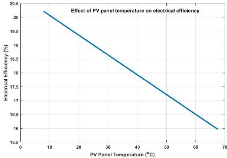
**Figure 7.3:** Effect of PV Cell temperatures on panel efficiency
