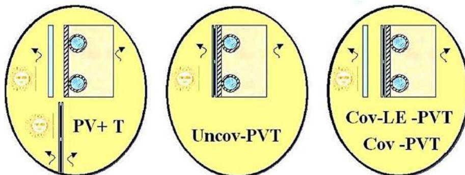
Figure 2.3: Water Based PVT Configurations studied by Fraisse et al. [28]
