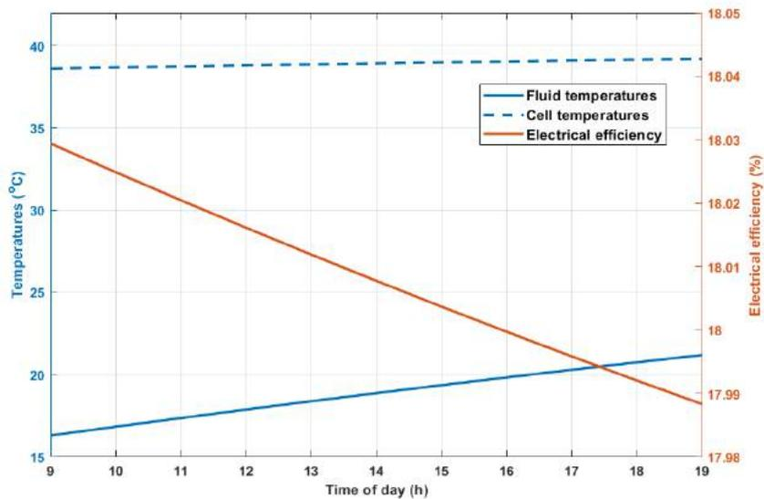
Figure 7.23: Averaged out fluid & cell temperature variations throughout the day, against electrical efficiency
