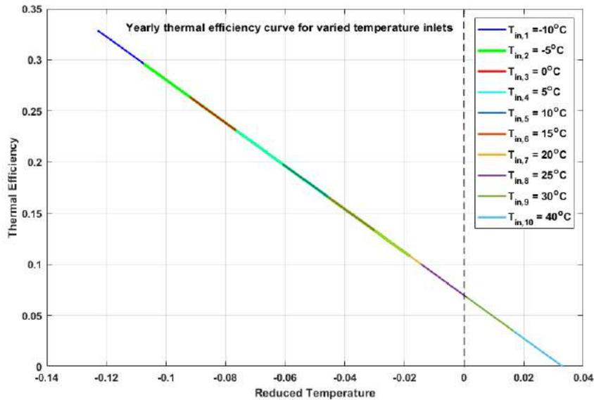
Figure 7.18: Thermal efficiency curves with varying inlet temperatures
