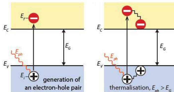
**Figure 1.1:** Photon Absorption illustration in a semiconductor, with bandgap  $E_g$  [42]
