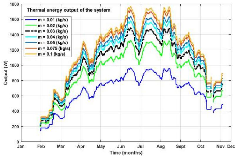
**Figure 7.16:** Characteristic thermal output for varying flow rates
