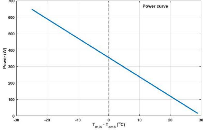
**Figure 7.8:** Power curve for the thermal collector
