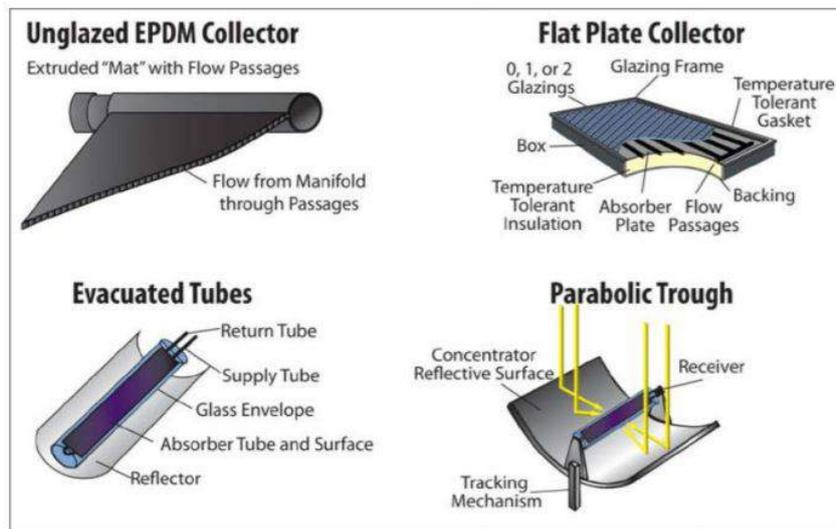
**Figure 2.1:** Primary solar thermal technologies [22]
