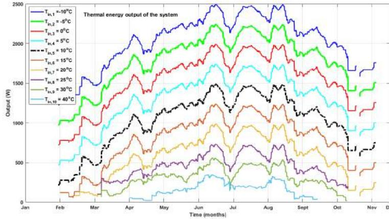
**Figure 7.19:** Characteristic thermal output for varying inlet temperatures
