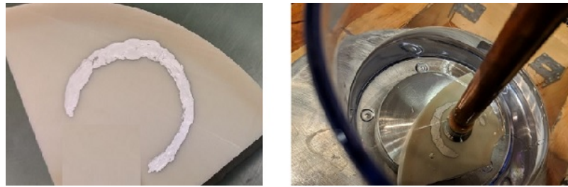
Figure 4.19: Experiment with conductive paint deposit on rubber sample
