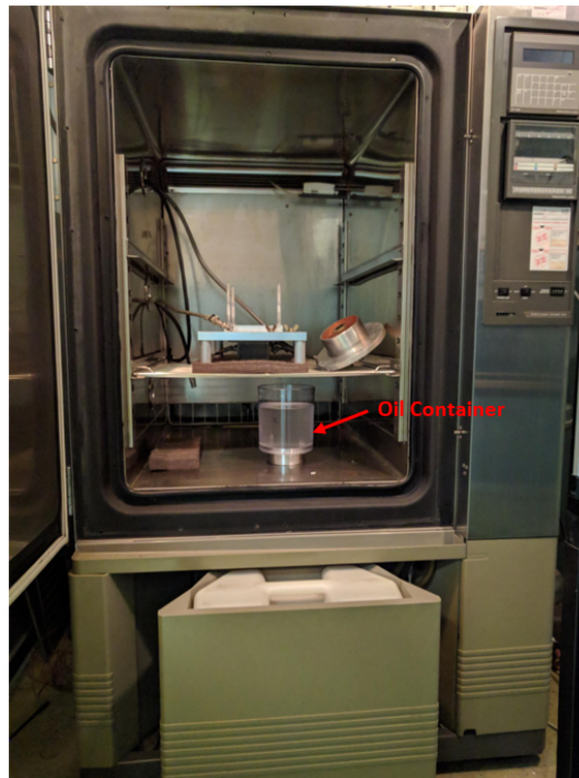
Figure 4.22: Climate chamber used for oil sample preparation of different moisture level (water activity)
