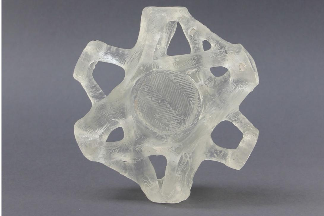
Topologically Optimised Cast Glass Grid Shell Node
