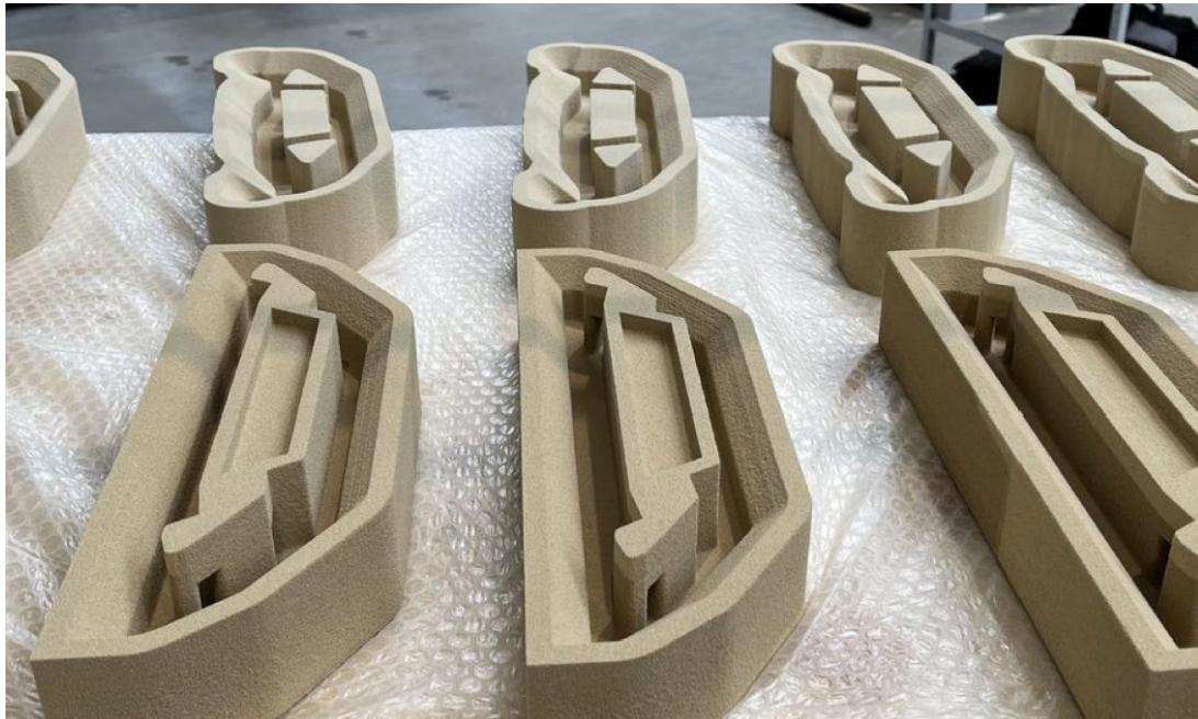
3D printed Sand Moulds
