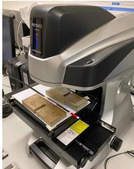
Figure 5.19: Setup used to take the tape surface image at the heated zone after the end of process location.
