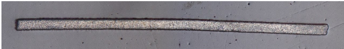
Figure 5.22: Tape cross-section profile for as-received tape.
