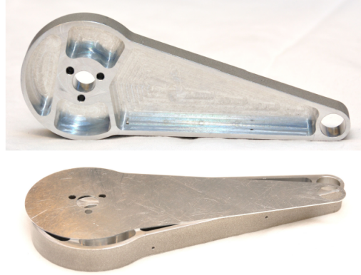
Figure 6.5: Lower limb pictures. In the upper picture the inner structure is clearly visible. In the lower picture also the cover plate is shown. The cover plate and the lower limb are glued together.
