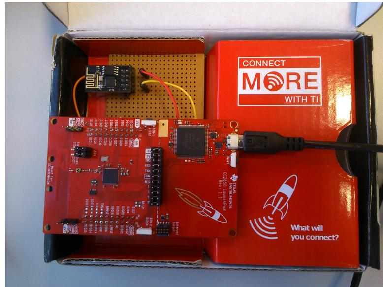
Figure 6.4: Concentrator node with CC2650 launchpad and ESP8266 WiFi module
