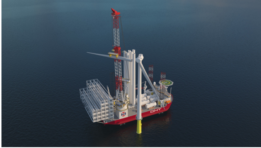
Figure 3.11: Render of a NG-20000X installing a wind turbine [20]
