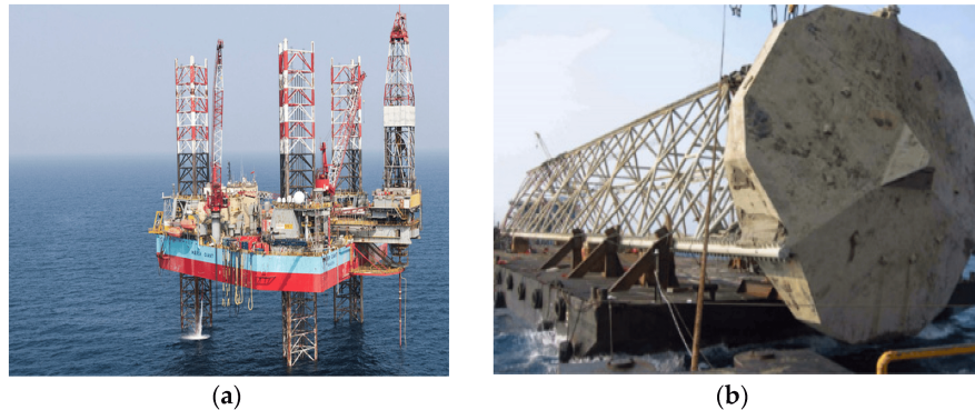
Figure 2.4: JU vessel (a) and spudcan (b)
