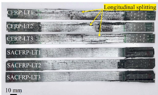
Fig. 8. Failure modes of the UD CFRP and SACFRP after longitudinal tensile tests.
