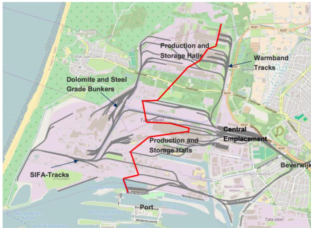
Figure 4.1: Map of the Tata Steel IJmuiden facilities, the red line is the non-physical separation of the west and central networks. On the west network (left) mainly raw materials and liquid steel are transported, on the central network (right) the various (semi-finished) steel products are transported. Source: Van der Linden (2018).
