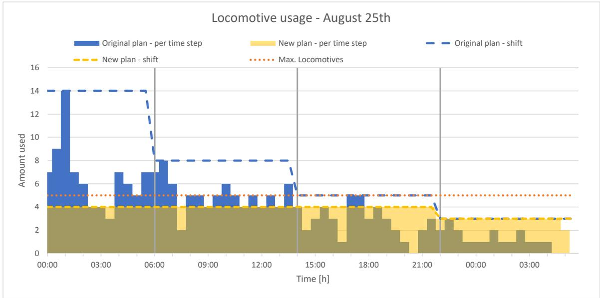
Figure G.7: Locomotive usage - August 25<sup>th</sup>
