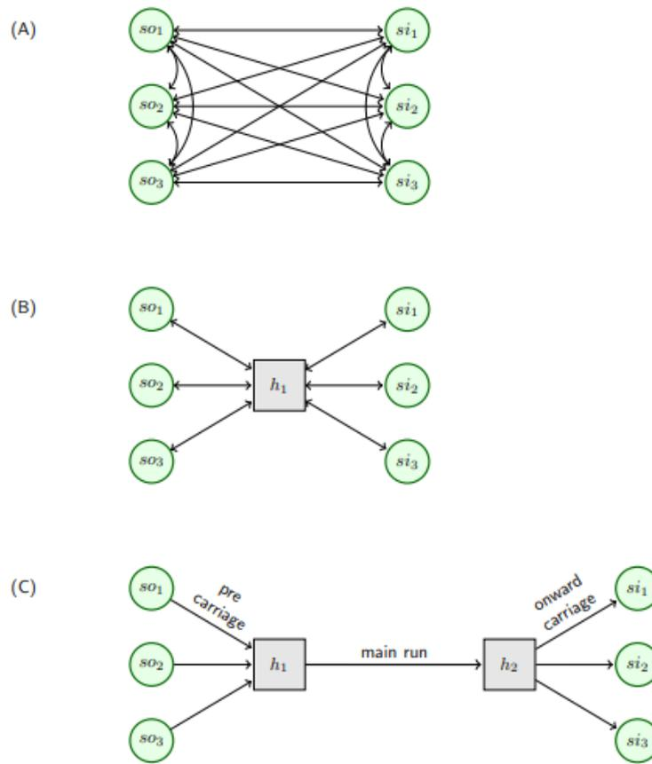
Figure 2.1: A: Point-to-point network, B: two-staged hub-and-spoke network, C: three-staged hub-and-spoke transport network, from (Schönemann, 2016)
