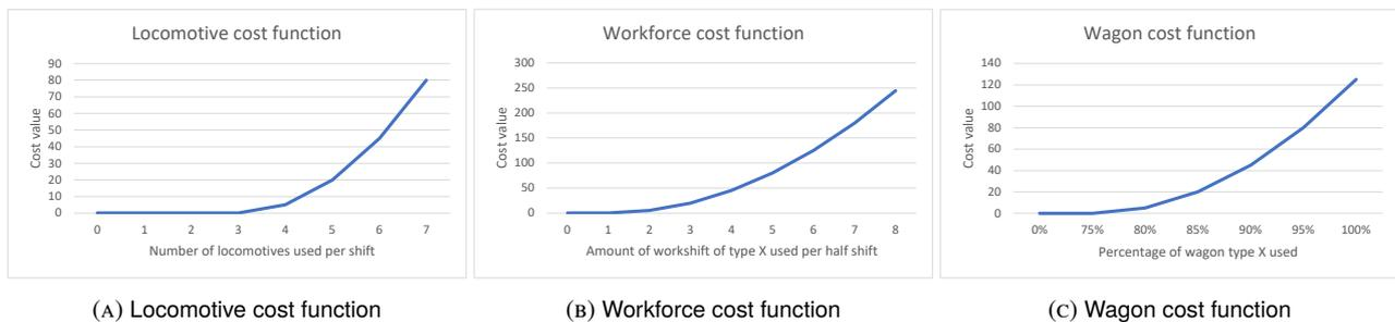
FIGURE 3: Cost functions for each of the KPIs
