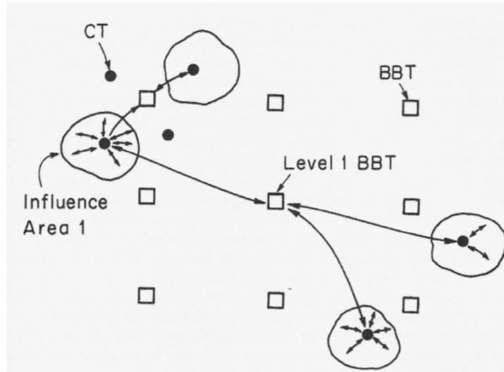
Figure 2.2: Consolidation and Break-bulk terminals in a many-to-many system (Daganzo, 2005)
