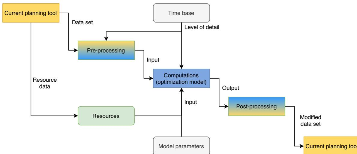
Figure 6.1: High level model architecture. Yellow = Planwise, Yellow/Blue = Excel & Python, Blue = Python
