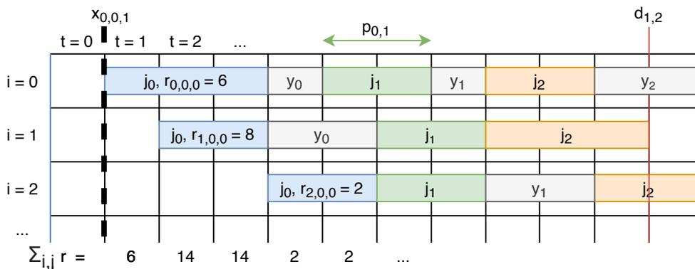
Figure 6.3: Example representation of a schedule including many of the variables, indexes and other parameters of the MILP model.
