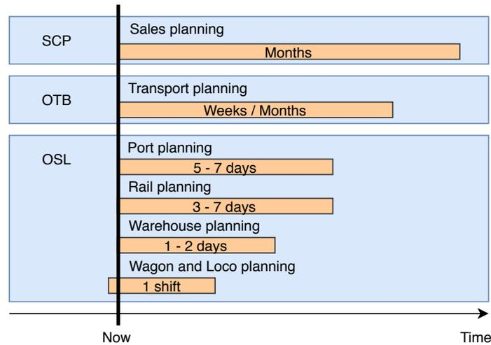
Figure 4.5: Current practice in the various levels of the planning process, SCP: Supply chain planning, OTB: Outbound department, OSL: On-Site Logistics department, adapted from Tata Steel (n.d.-b)
