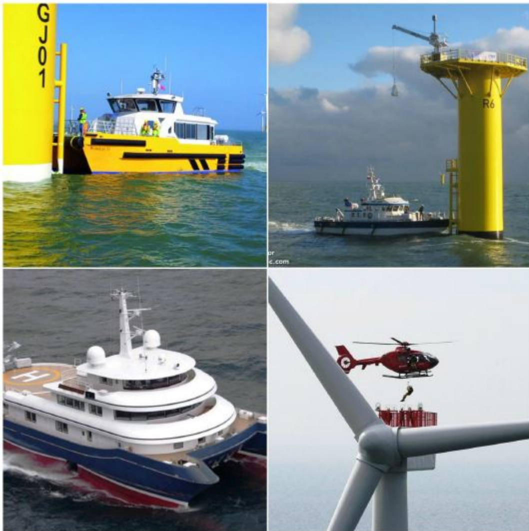
Figure 1.4: Examples of different offshore access systems; clockwise: Windcat workboat, Fob Lady, SWATH and helicopter .
