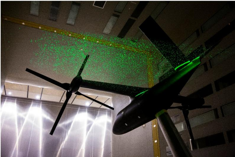
Figure 8-6. The extent of the HFSB stream tube that is captured within the laser sheet. The FoV was 1.1×1.1 m<sup>2</sup>.
