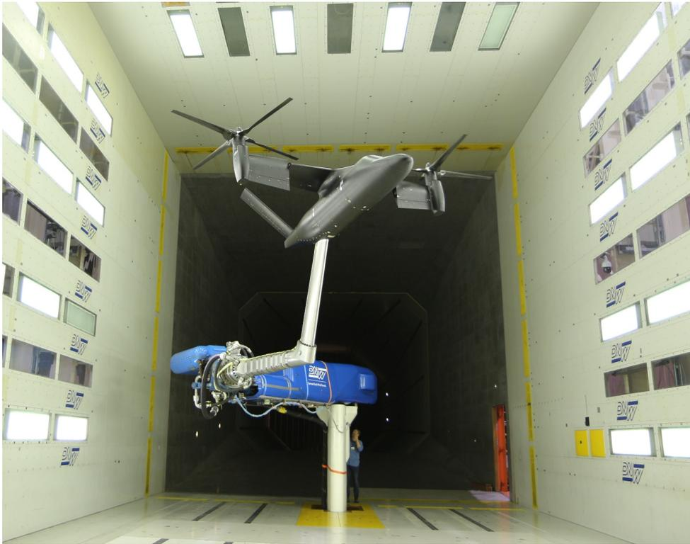
Figure 8-2. The NEXTTRIP tiltrotor aircraft installed in the DNW-LLF  $9.5 \times 9.5 \text{ m}^2$  test-section.
