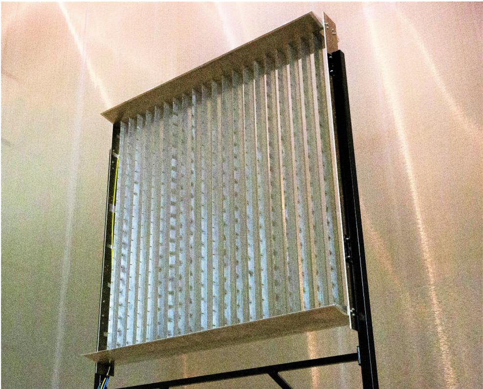
Figure 8-4. NLR seeding rake of 400 bubble generators, 20 wings and cross-section area of 9m<sup>2</sup>, installed in the DNW-LLF settling chamber.
