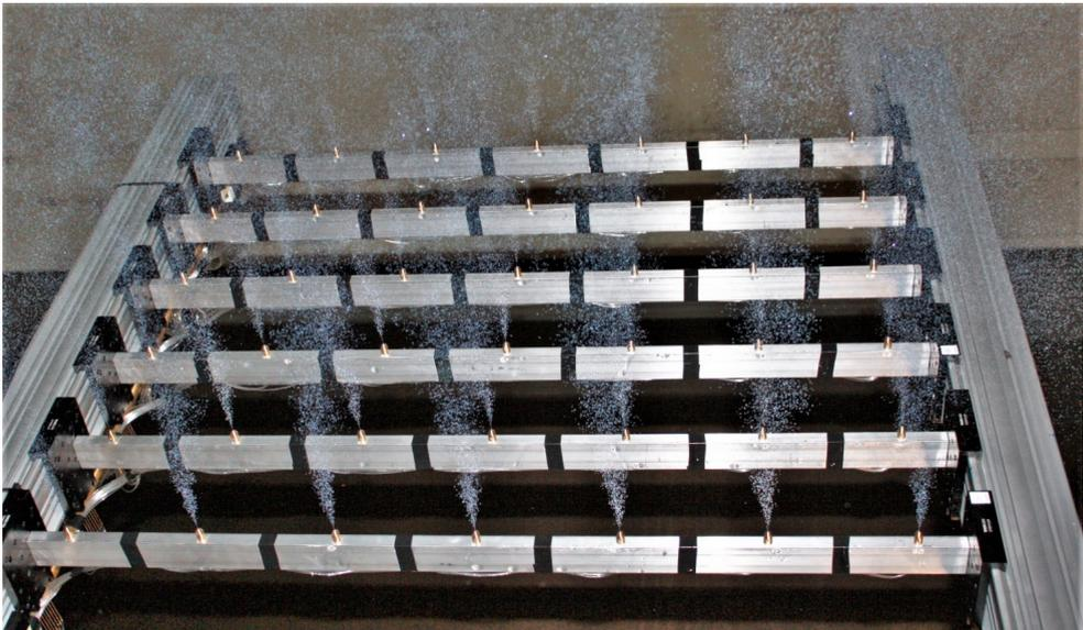
Figure 6-13. NLR's seeding rake of 42 bubble generators.
