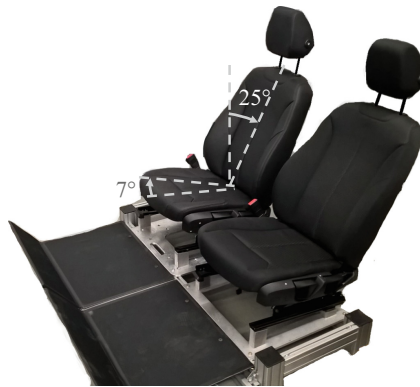
Fig. 1. Setup of the experiment. Leather and fabric seat mounted next to each other in the H-Point-Position
