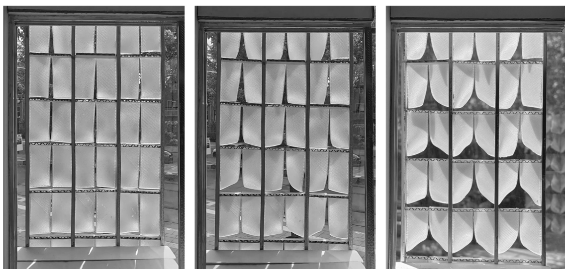
Figure 53 Panels changing from closed state to open state.
