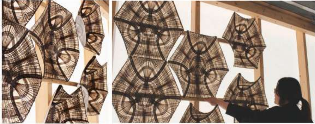
Figure 28 Thermo-fold self-adaptive biocomposite SMP façade. (Hassan et al., 2025)
