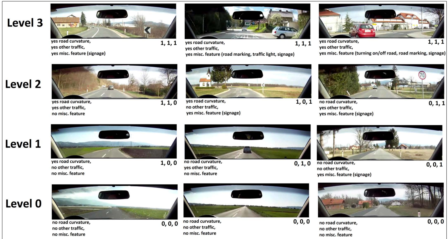
Figure 4: A dozen examples out of the full set of 60 to illustrate the grouping levels of complexity factors. The first factor pertained to road curvature, the second factor to other traffic, and the third factor to any combination of miscellaneous infrastructure/behavior, that is, road markings (excluding lane boundaries), multi-lane roads, signs/signals facing the driver, traffic lights, lane changes (self/other), and turning on/off road (self/other) [18].
