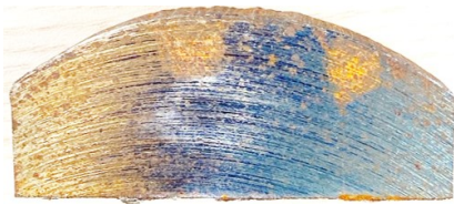
Fig. 13. Discolouration of cutting surface of a test piece due to improper cooling (test 8)
