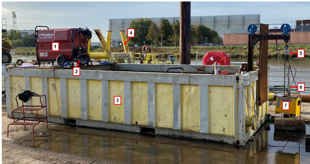
Figure 3.2: Test set-up: (1):DSW 1510-CA sawing machine from Hilti (2):Tachometer (3):Steel container (4):Diamond wire (5):Hand hoist (6):Load cell (7):(variable) test weight
