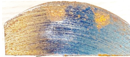
Figure 4.14: Under nominal test conditions, but with improper cooling, discolouration of the cutting surface was observed on a round S235 test piece (d: 120mm, h: 100mm)
