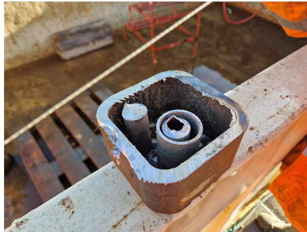
Figure 4.24: Cut test piece consisting of a tube (120x120x100mm, thickness 16mm) containing loose round pieces
