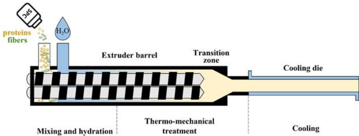
**Figure 1:** Diagram illustrating the steps of high-moisture extrusion involved in the production of plant-based meat alternatives. *Credit: Ekaterina D. Garina, adapted from [Garina et. al 2024](#) under [creative commons 4.0 license](#).*
