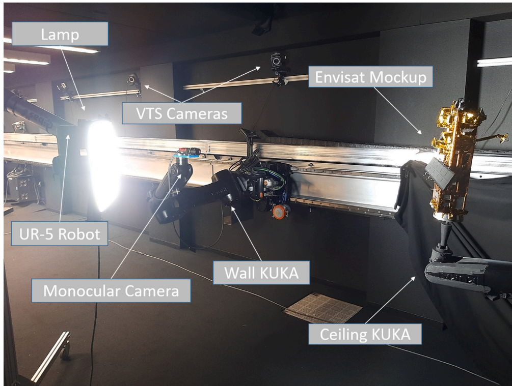
Fig. 3. GRALS testbed with the scaled 1:25 Envisat mockup mounted on the wall KUKA, the VTS and the monocular camera mounted on the ceiling KUKA. Two of the VTS cameras and the Sun lamp are also shown.
