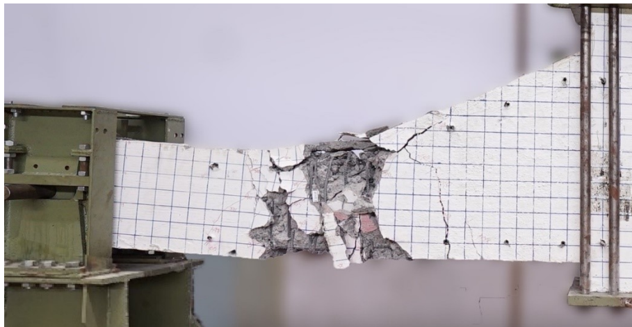
(a) Failure pattern of haunch-strengthened beam-to-column joint.
