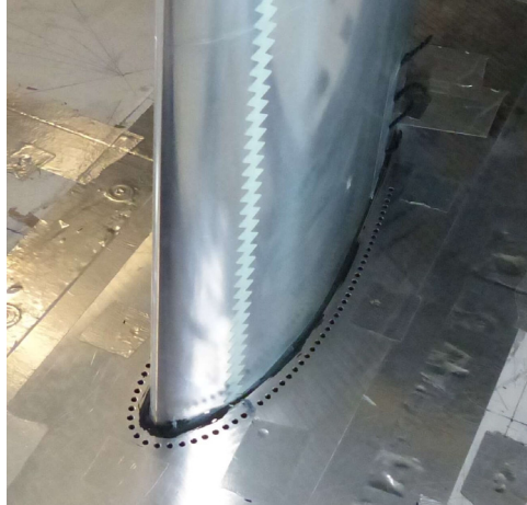
Figure A.3: Holes in the side plate around the main element of the wing for the suction system.
