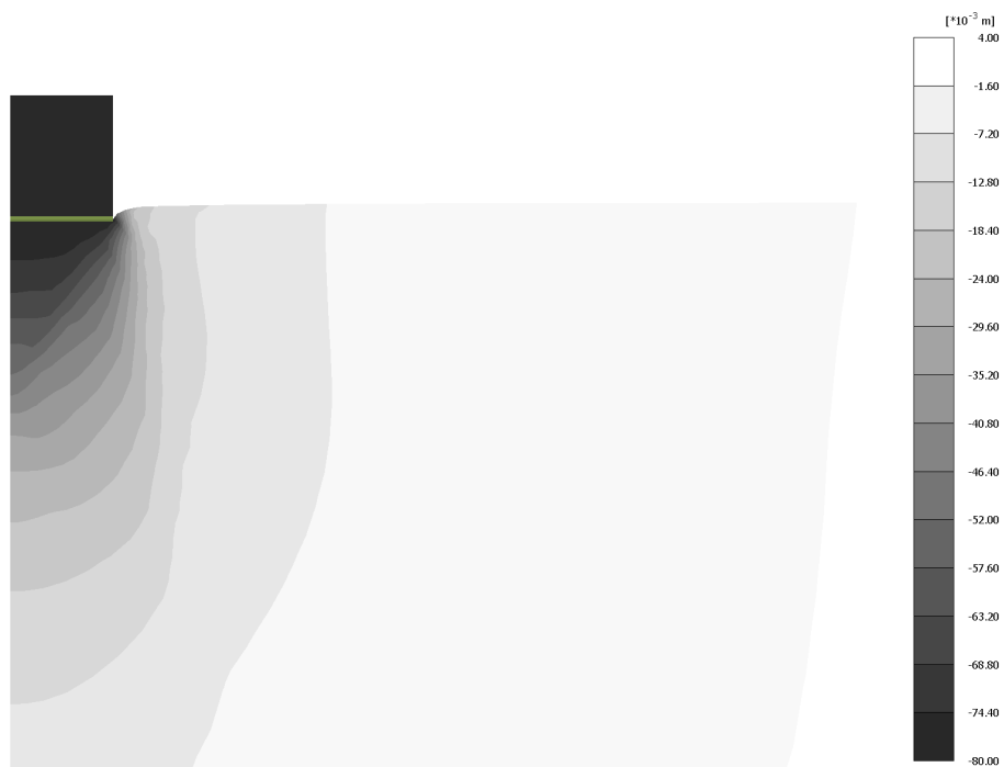
Figure D.3: Distribution of vertical displacements at the foundation.
