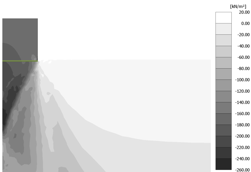
Figure D.1: Vertical Stress distribution after the first load peak on the foundation (164 kPa)
