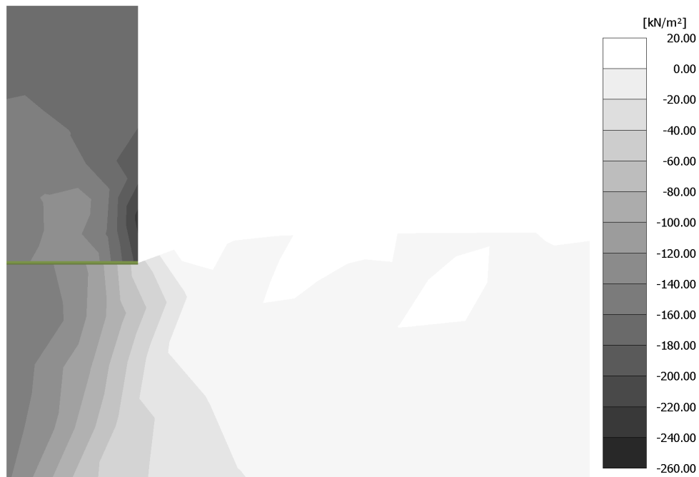
Figure D.2: Detailed close-up of the vertical stress distribution near the foundation corner in Figure D.1
