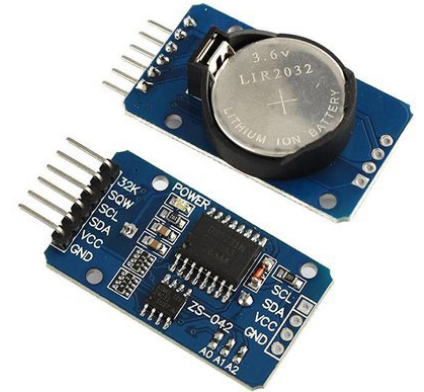
Figure 4.7 RTC module with cell battery
