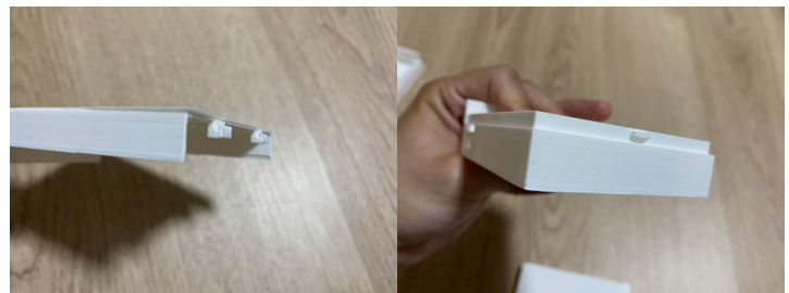
Figure 6.21 Failed printed snap-fit joints
