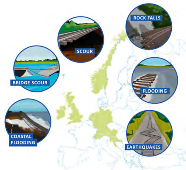
Fig. 1. Different types of failure on railway infrastructure [10]
