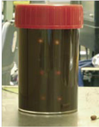
Figure 1.1. Demonstration of the MDS principle. The lightest plastic balls float near the top and the heavier ones float deeper, i.e. closer to the magnet surface. The opaqueness of the ferrofluid is the reason for ultrasound imaging [W2Plastics 2008].
