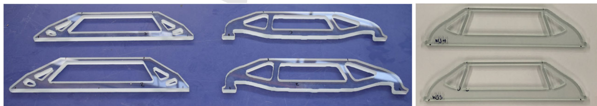
Figure 1.9: Images of fabricated waterjet cut float glass beam specimen. The volume-based is on the left, the stress-based is in the middle, and the stiffness-based is on the right, on a separate photo. (Jewett et al., 2024)
