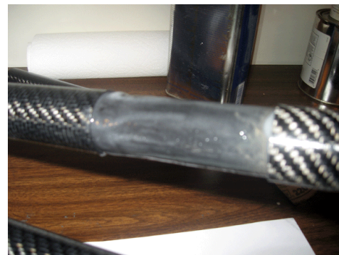
Figure 21.4: Clarifying picture for epoxy adhesive bonding [65]
