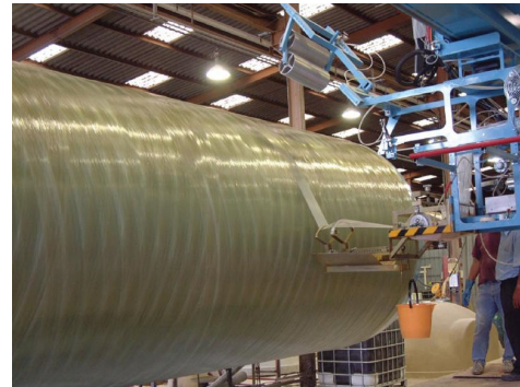
Figure 21.2: Large circular product made using filament winding [63]
