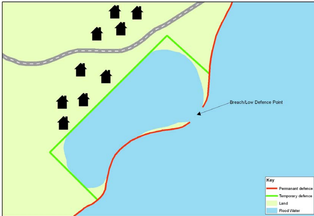
Figure 5.14b Plan view example of use of a temporary system to contain flood water
