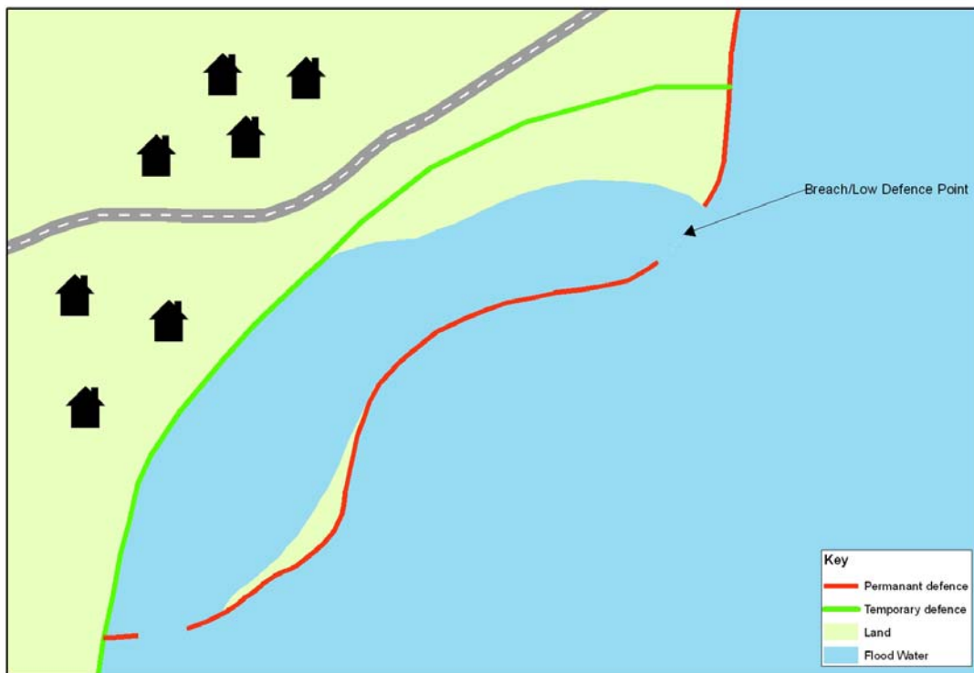
Figure 5.15 Plan view example of use of a temporary system to divert and direct flood water
