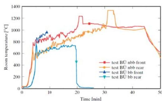
**Figure 3-14: Ceiling room temperatures in tests BU nbb and BU bb**
