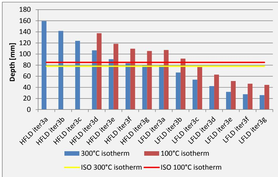
Figure 7-40: Charring depth and unaffected depth compared – unprotected
