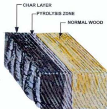
Figure 3-5: Illustration of charring of wood section
