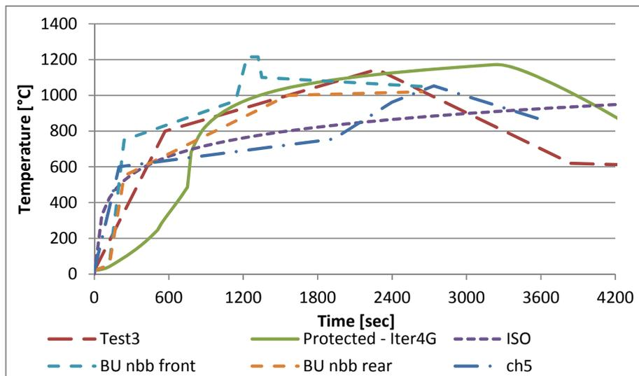
Figure 7-42: Temperature curves for protected fire room
