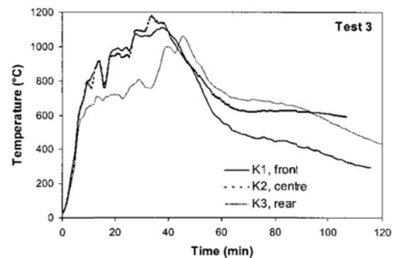
Figure 3-13: Room temperatures for test 3 (protected)
