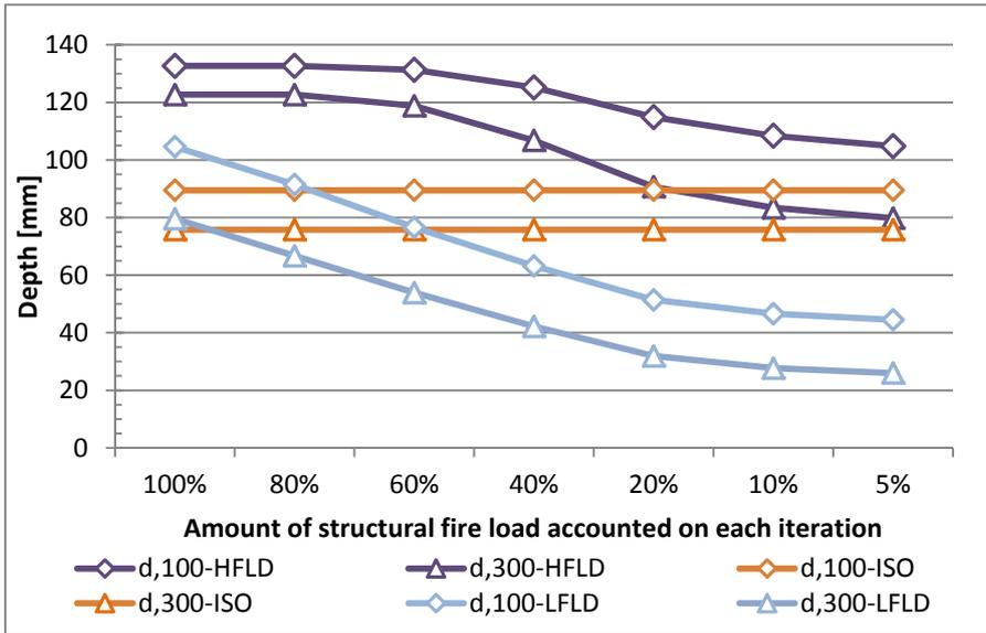
In the graph beside, the depth for the 300°C and the 100°C isotherms are given for three fire exposures, namely: the ISO fire curve (orange lines), the High Fire Load Density (violet lines), and the Low Fire Load Density (sky-blue lines). All these values are obtained at 120 min. As it is shown, for the highest fire load density, the distance between the violet lines is reducing. It is due to the fire period and it is explained in more details below.
