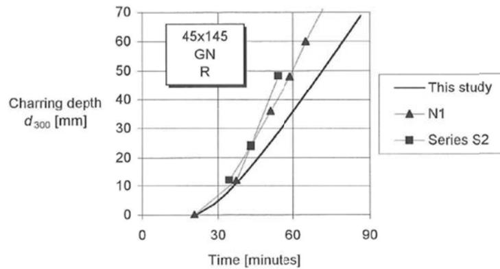
Figure 7-18: Charring depth versus time - Comparison of calculated values with test results for one layer of gypsum plasterboard GN, failure time 20 min – From (94)
