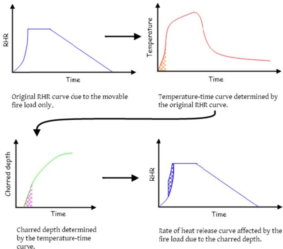
Figure 7-10: Suggested fire model in unprotected timber compartment
