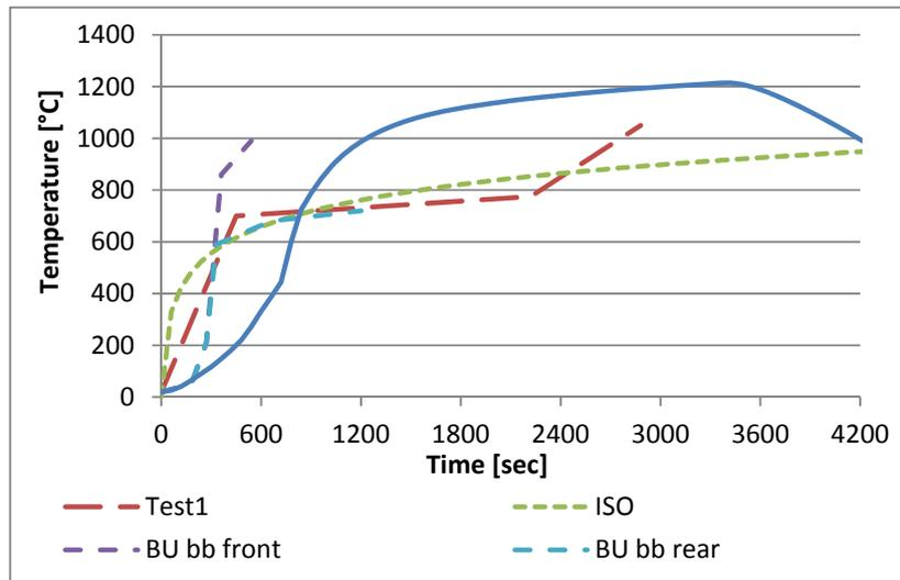
Figure 7-43: Temperature curves for unprotected fire room configuration
