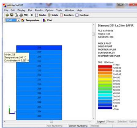
*Depth of the 100°C isotherm according to finite thermal analysis for the high initial fire load density with an unprotected fire compartment. It worth noting that the fire curve has its maximum temperature of approximately 1300°C at 8340 sec (2h19min).*
