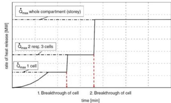
Figure 7-7: Development of RHH during spreading of fire through the compartment (qualitative) (81)
