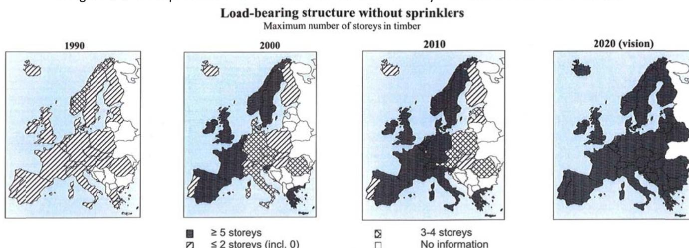
Figure 2-1: Changing in restrictions on Load-bearing structure without sprinklers (6)
