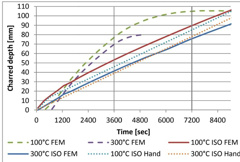
*In the graph beside, the depth for the 300°C and the 100°C isotherms are given for different fire exposures. Natural fire curve, HFLD-Iter3G (dashed lines), ISO fire exposure computed by finite element analysis (solid lines), and for an ISO fire exposure computed by formulas in EN1995-1-2 (dotted lines).*
