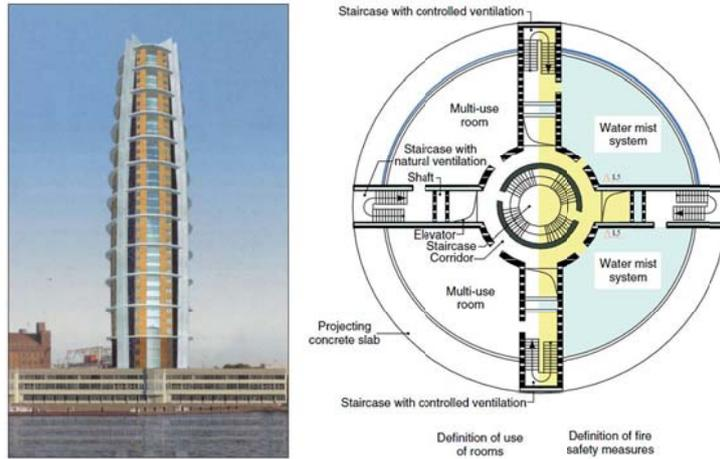
Figure 5-9: Technical feasibility of high-rise timber structure, Dock tower
