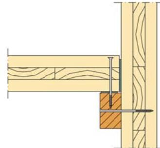
Figure 6-5: Balloon frame connection, from (77)
