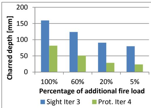
In Figure 7-31, it is shown the charred depths for the in-sight (blue) and protected (green) element. As can be seen, the protected configuration has the lower charred depth.
