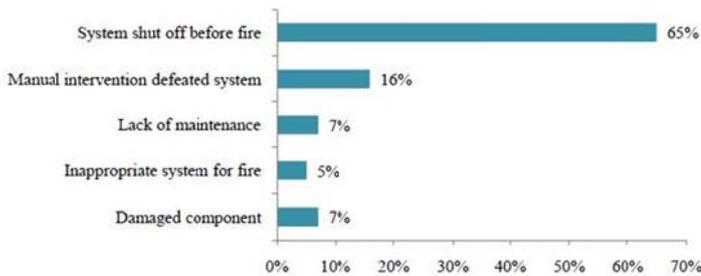
Figure 4-2: Reasons When Sprinklers Fail to Operate, 2005-2009
