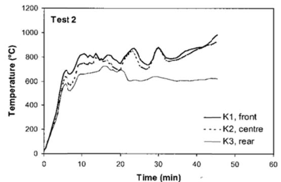
Figure 3-12: Room temperatures for test 2 (protected)
