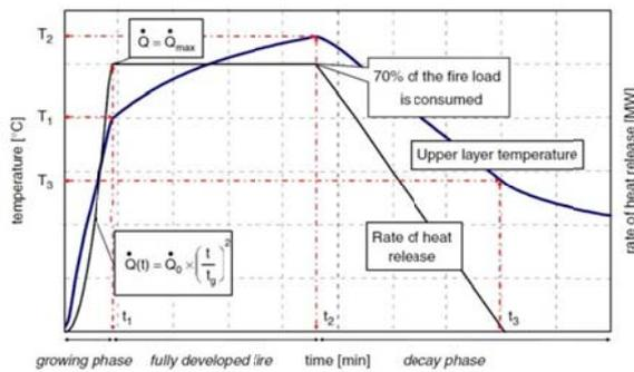
Figure 7-6: iBMB parametric curve and HRR (81)
