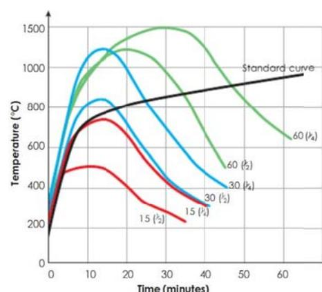
**Figure 7-4: Time-temperature curves based on different opening factors and different load density (kg(opening factor))**
