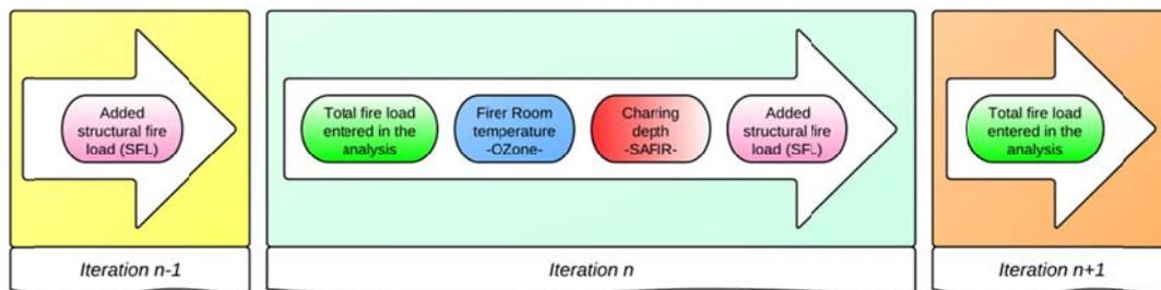
**Figure 7-12: Detailed view of steps involved in each iteration**
