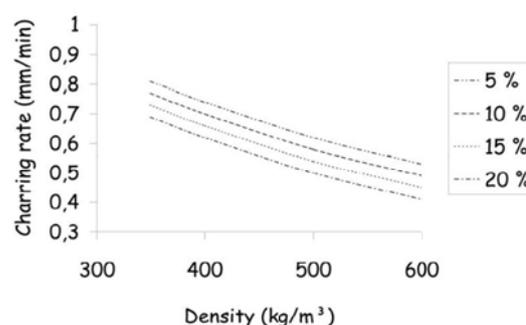
Figure 3-1: Charring rates as affected by density and moisture ratio (33)
