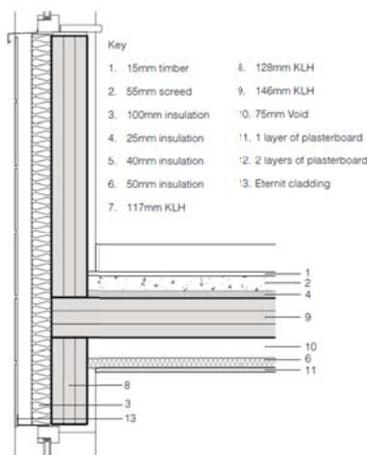
Figure 5-3: Element's dimensions in Murray Grove timber building
