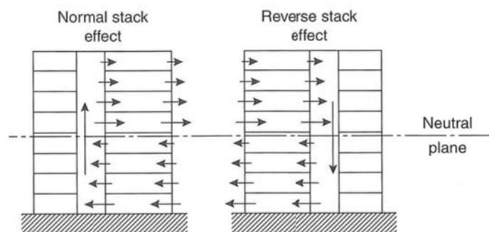
Figure 4-1: Air movement due to stack effect and reverse stack effect
