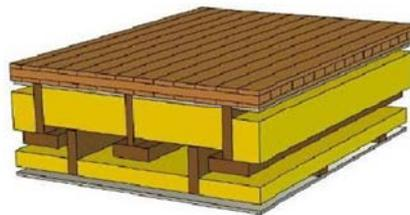
Figure 6-10: Limnologen floor element, please note the floor slab with the T-beams
