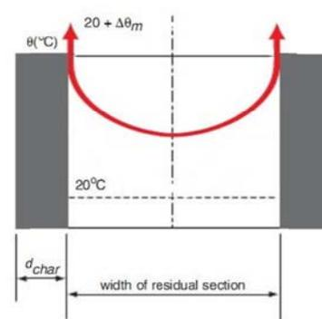
Figure 3-3: Temperature profile for thickness smaller than the minimum, thermally thin sections
