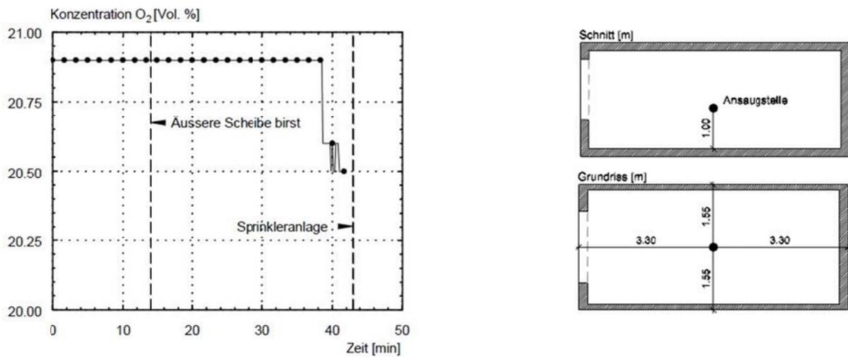
Figure 3-4: Oxygen depletion during fire test BU nbb (no gypsum protection)
