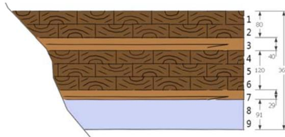
Figure 6-16: CLT 360 mm residual section, a depth of 91 mm is affected by fire
