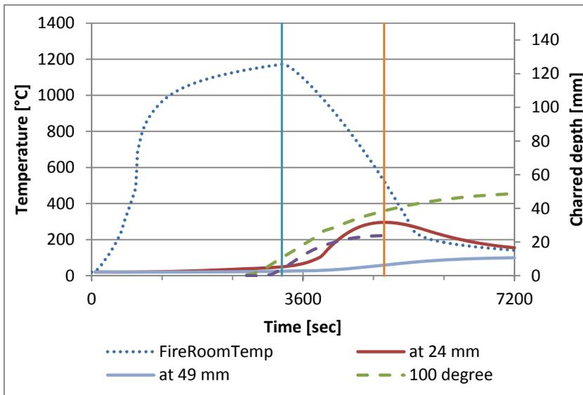
Figure 7-35: Time lag between the maximum fire room temperature and the charred depth (protected configuration)
