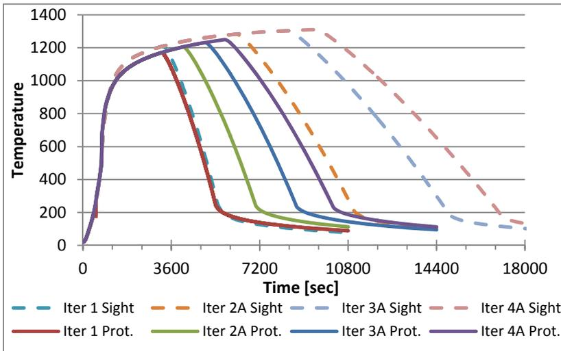
In the figure beside the different fire curves for the protected (solid lines) and unprotected (dashed lines) configuration are shown.
