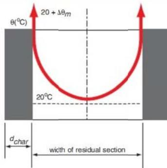
Figure 3-2: Temperature profile for thickness greater than the minimum, thermally thick sections
