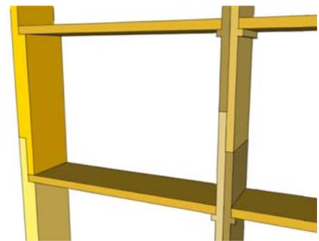
Figure 6-3: Connection proposed
