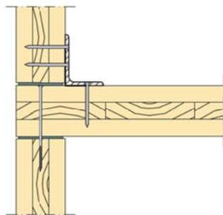
Figure 6-4: Platform frame connection from (77)
