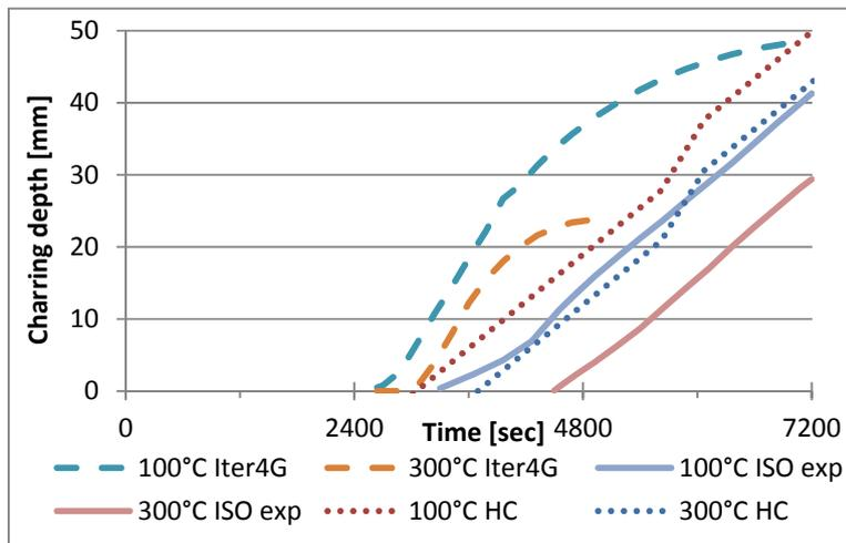
*In the figure beside the 100°C and 300°C isotherms are shown for a natural fire exposure, according to natural fire curve, Iter4G (dashed lines), for an ISO fire exposure computed by finite element analysis (solid lines), and for an ISO fire exposure computed by formulas in EN1995-1-2 (dotted lines).*
