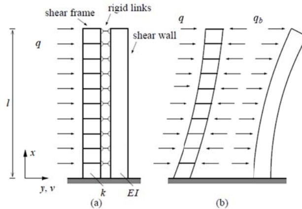
Figure 6-15: Shear beam-bending beam system
