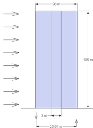
Figure 6-2: Side view of the building with wind load and restoring forces
