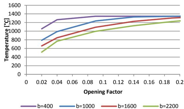
Figure 7-5: Parametric fire curves from EC5 depending on the thermal boundaries and the opening factor (gypsum plaster board  $b = 410 \text{ W s}^{1/2}/\text{m}^2\text{K}$ , normal weight concrete  $b = 1900 \text{ W s}^{1/2}/\text{m}^2\text{K}$ )
