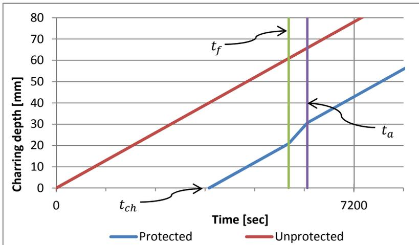
Figure 7-11: Charred depths according to standard fire curve (ISO)
