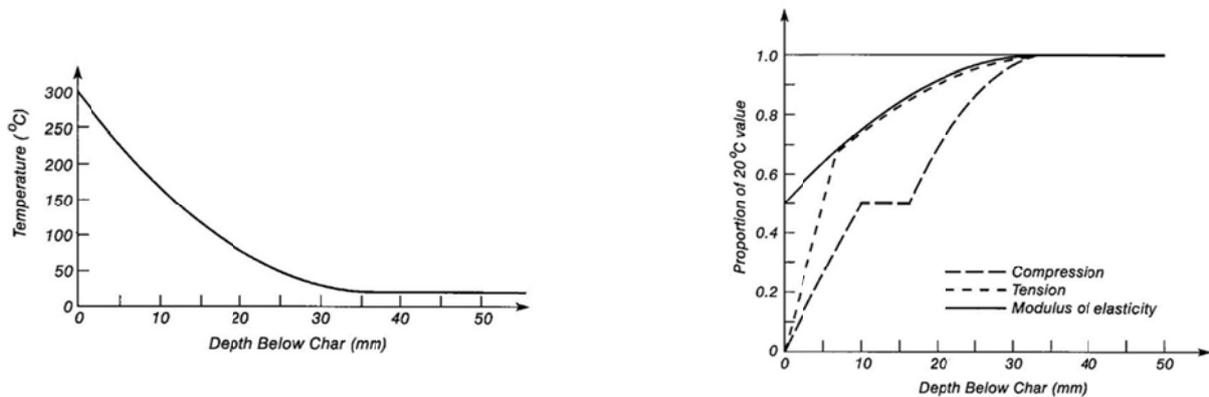
Figure 3-6: Temperature profile (left) and Residual properties (right)
