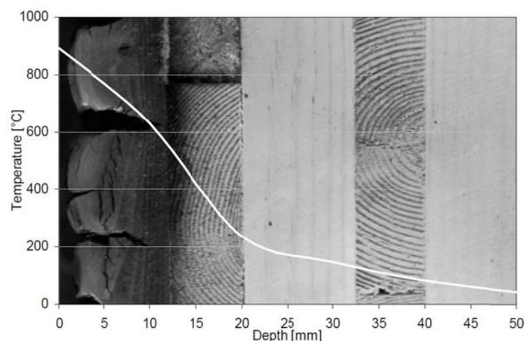
**Figure 3-7: Step temperature gradient in the heated zone of the wood (33)**
