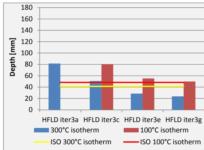
Figure 7-41: Charring depth and unaffected depth compared – protected
