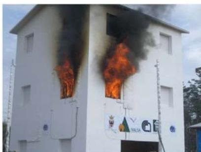
**Figure 3-8: Full scale test after 40 minutes (flashover)**
