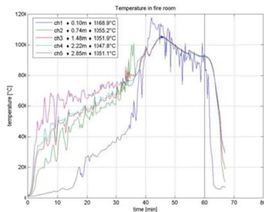
Figure 3-10: Fire room temperatures at different heights
