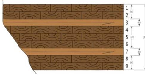
Figure 6-14: CLT 360 mm section, 9 layers 40 mm each
