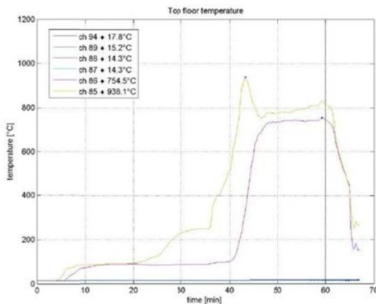
Figure 3-9: Temperatures across the ceiling thickness
