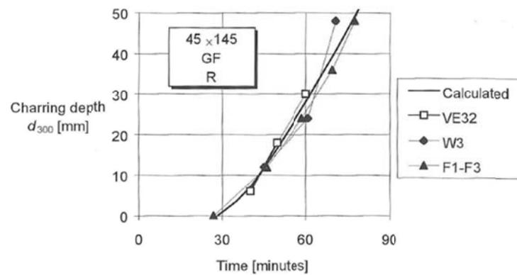
Figure 7-19: Charring depth versus time - Comparison of calculated values with test results for one layer of gypsum plasterboard GF, failure time 28 min - From (94)
