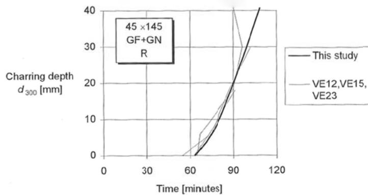
Figure 7-20: Charring depth versus time - Comparison of calculated values with test results for two layers of gypsum plasterboard GN+GF, failure time 64 min – From (94)
