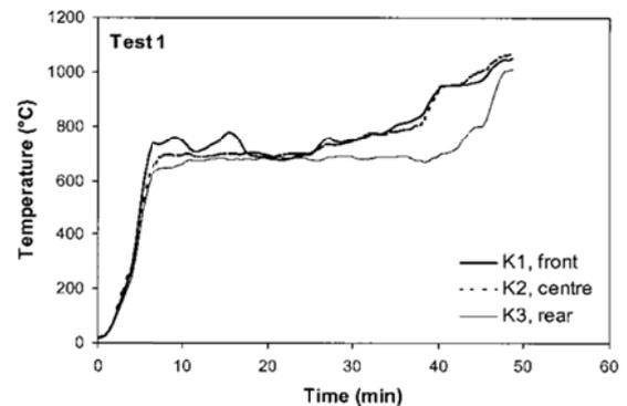
Figure 3-11: Room temperatures for test 1 (no gypsum)
