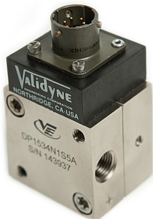
Figure 7: The differential pressure sensor that was used in the current test setup to control the tunnel free-stream inlet velocity.
