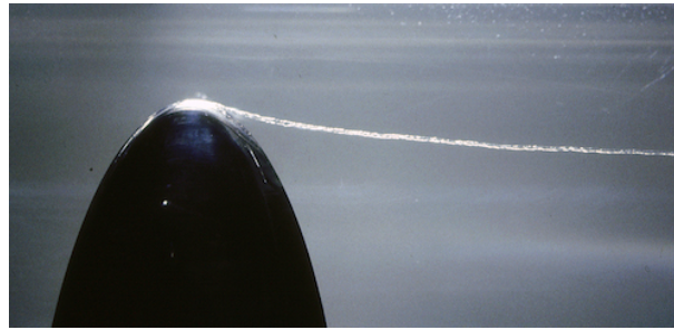
Figure 1.4: Photograph of an isolated cavitating tip-vortex behind the hydrofoil. Flow direction is from left to right. [4].
