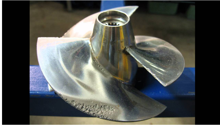
Figure 1.2: Photograph of a propeller showing the erosion of material on surface[2].
