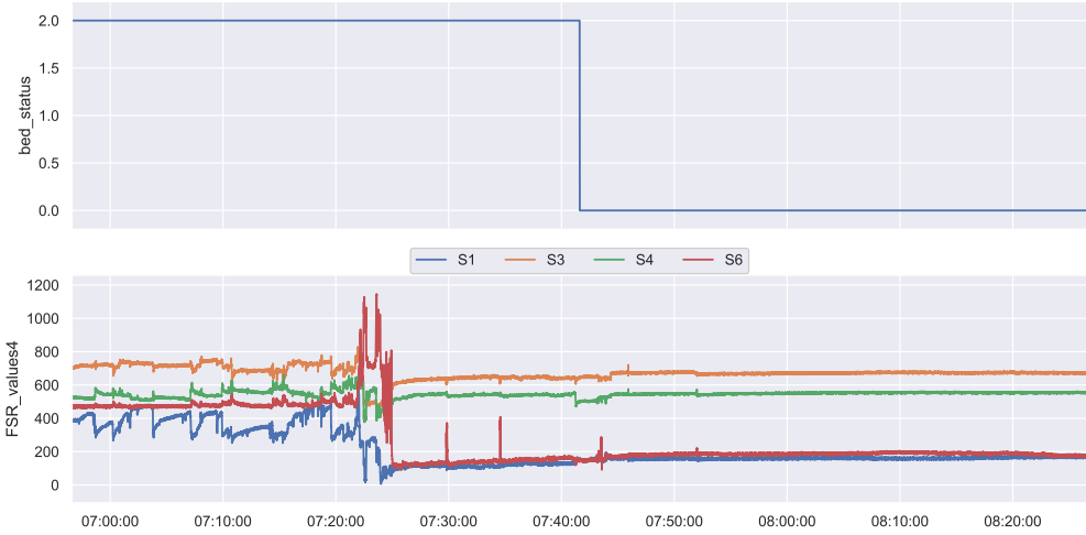
Figure A.7: Visualisation of a bed exit of another client who is at higher risk of falling
