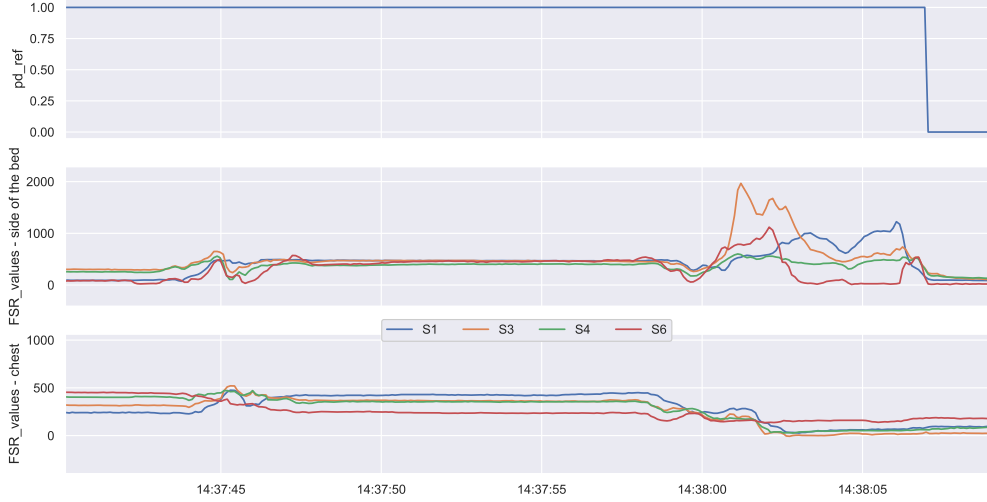
(b) Setup 2: Rolling to the right side of the bed, sitting up then leaving the bed
