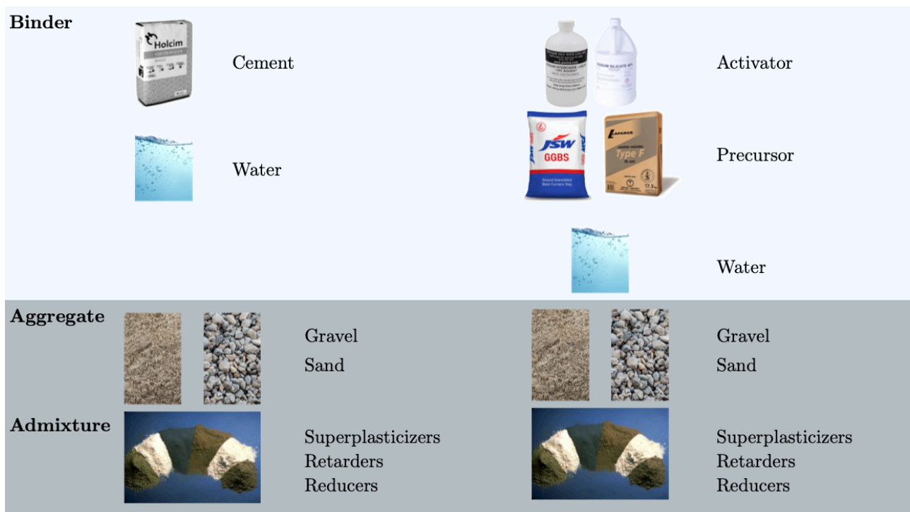
Figure 2.1 - Regular (left) and alkali activated (right) concrete components (self-made)
