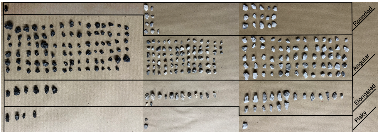
Figure 4.3 - Shape test results, from left to right: copper slag, secondary aggregate, blast furnace slag
