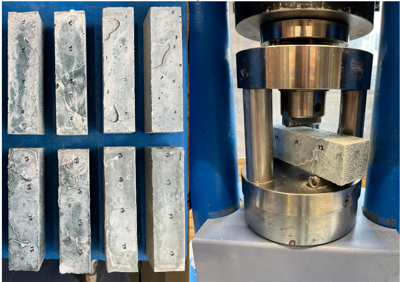
Figure B.3 - Flexural strength test setup
