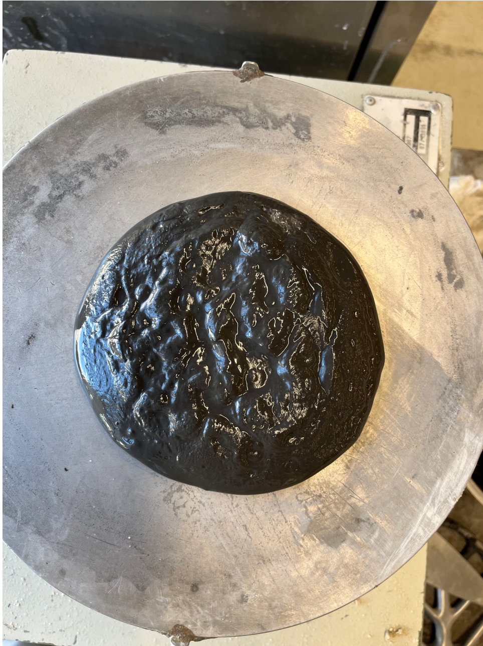
Figure B.9 - Workability test of Paste trial mix 6
