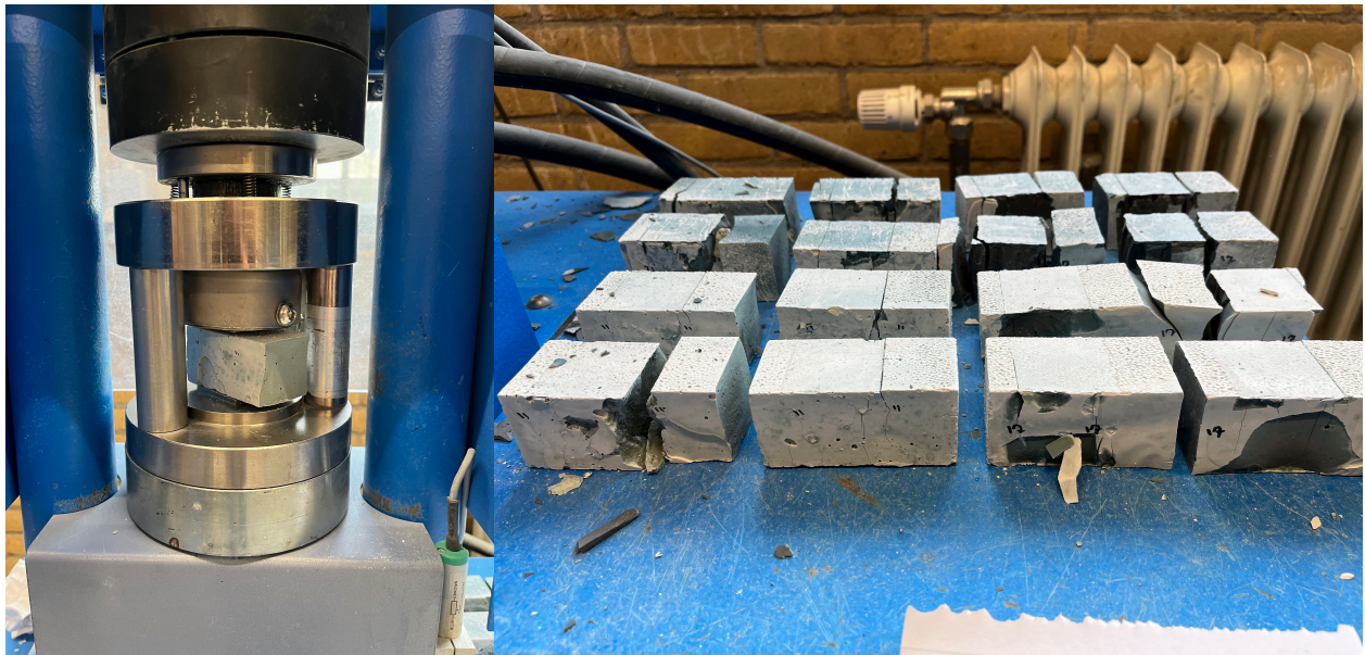
Figure B.5 - Compressive strength testing setup (left) and failed specimens (right)
