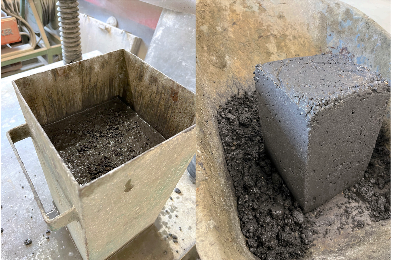
Figure E.3 - Results of workability of CT04
