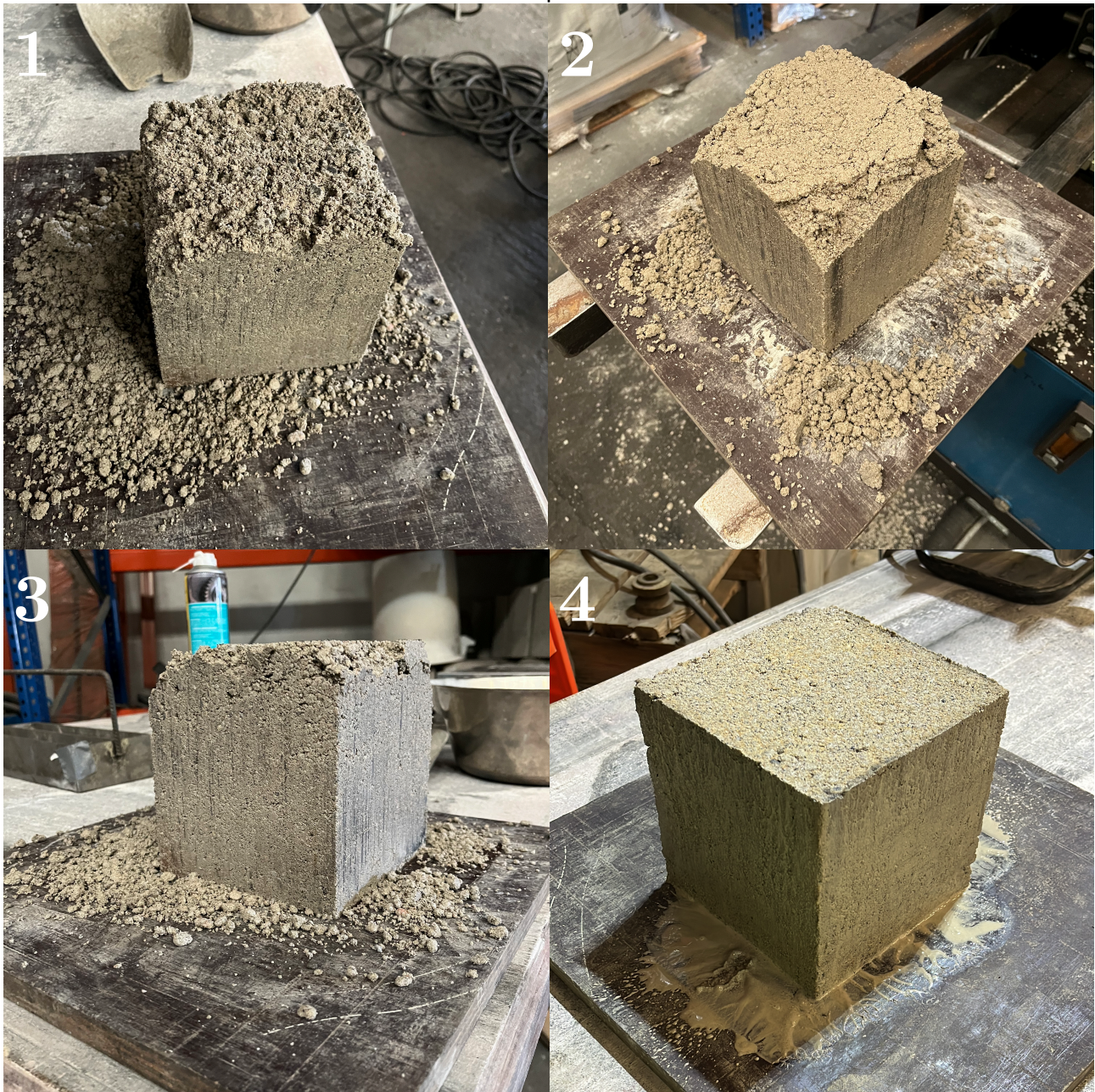
Figure E.4 - Workability results from small compaction machine
