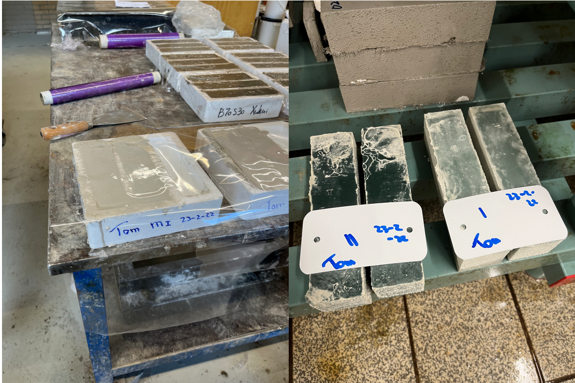
Figure B.2 - Preparation of paste in molds (left) and specimens in curing room (right)
