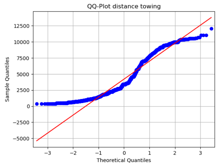
Figure A.12: QQ-plot aircraft taxi-distance towing
