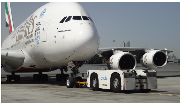
Figure 4.3: Towing operation using external tow-bar [13]
