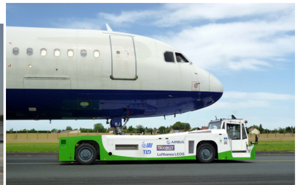
Figure 4.4: Towing operation using TaxiBot [14]
