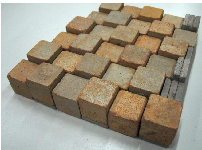
Figuur 2.1: modelschematisering steenzetting in dambord patroon
