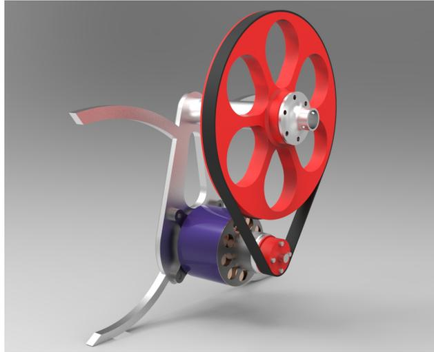
Figure 3.10: A CAD generated design of the drivetrain layout. The large gear ratio is clearly visible. The part of the drivetrain shown here will be located inside the fairing.
