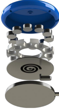
(a) An exploded view of the updated DAS-Actuator with the magnet-array and spiral groove visible.
