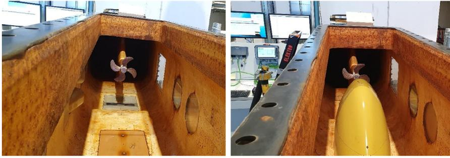
Figure 6.2: Cavitation tunnel set up. Left: Open water, Right: with wake generator. [45]
