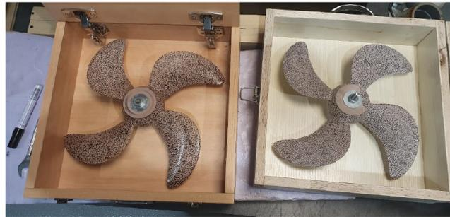
Figure 6.3: Model propeller for SikaBlock M700 propellers, with black markings. [45]
