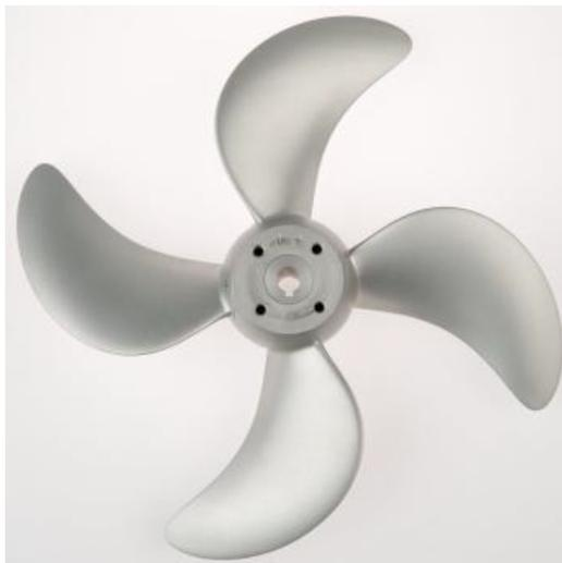
Figure 4.1: A wageningen c4-40 propeller with  $P/D_{0.7R} = 0.8$ , Source: MARIN. [42]
