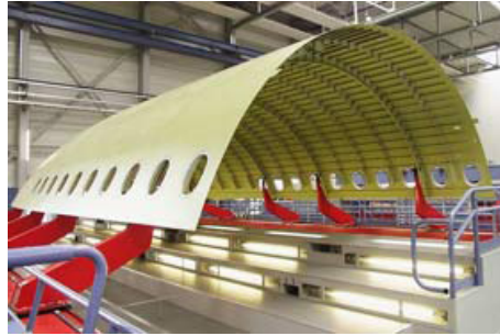
Figure 1.2: GLARE panel used in the upper part of the fuselage of the Airbus A380 (reprinted from [40]).
