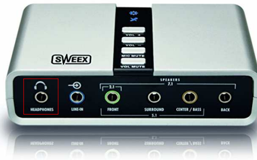
Figure 4-5: Front view of the Sweex SC016 16-bit sound card. The headphones connection (indicated by the red rectangle) is the output port that will be connected with the class D amplifier. The side of the sound card (not visible in this picture) contains the microphone port.
