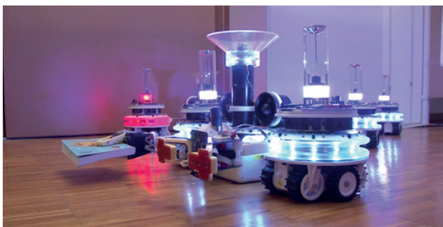
▲ Figure 2.9: The legs and grab robots of the Swarmanoid.
