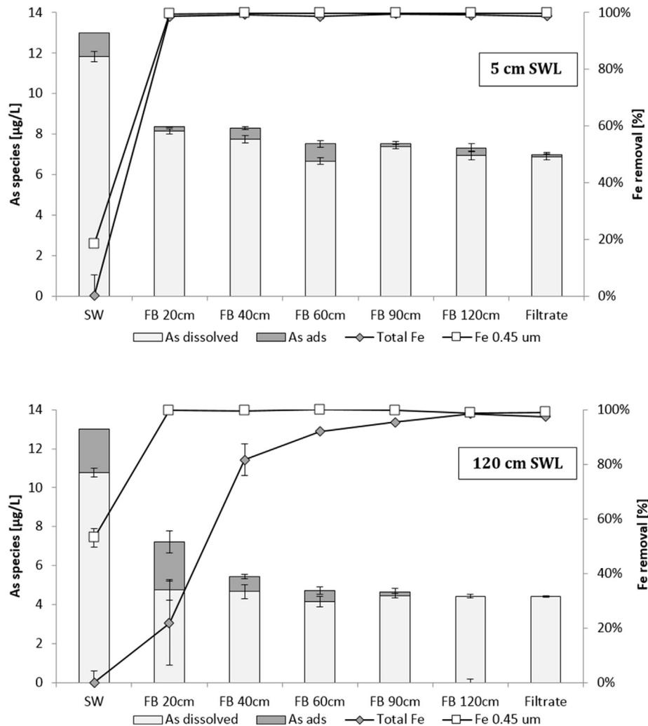
**Fig. 7.** Dissolved As and adsorbed As to mobile HFO (yet to be retained by the sand filter) in  $\mu\text{g/L}$ . On secondary axis Fe removal both over the filter bed depth (FB) at 5 cm SWL (top) and 120 cm SWL (bottom). Filtration velocity 1.5 m/h. Data shown are averaged values of week 6 and 7 of operation.
