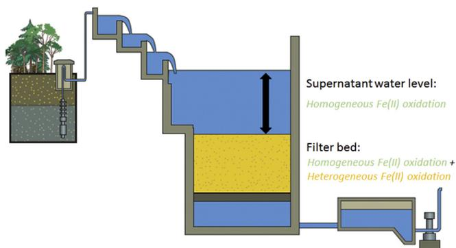
**Fig. 1.** Groundwater treatment: abstraction, followed by aeration and rapid filtration. Increasing the supernatant level, increases the amount of HFO entering the filter bed by lengthening residence time in the SWL.
