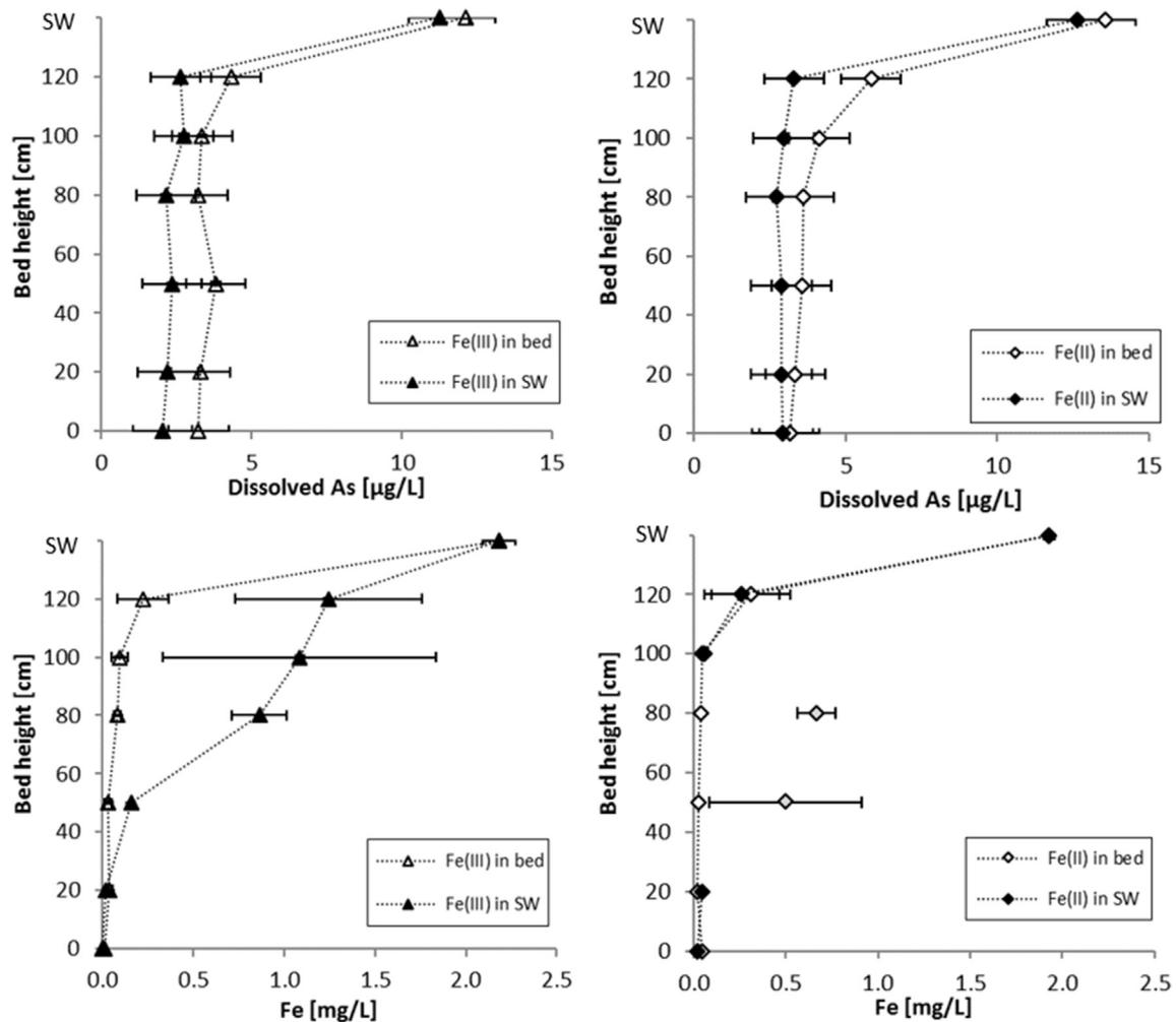
**Fig. 10.** Fe(III) (left) and Fe(II) (right) addition of 1 mg/L in supernatant water and filter bed at 110 cm bed height. All experiments were performed with 50 cm SWL and filtration velocity of 5 m/h.
