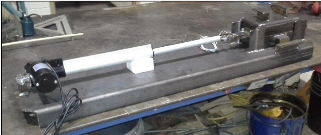
Figure 7. Final design of the adhesive test set-up
