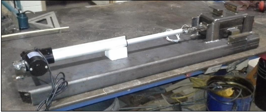
Figure 3.7 – Final design of the adhesive test set-up
