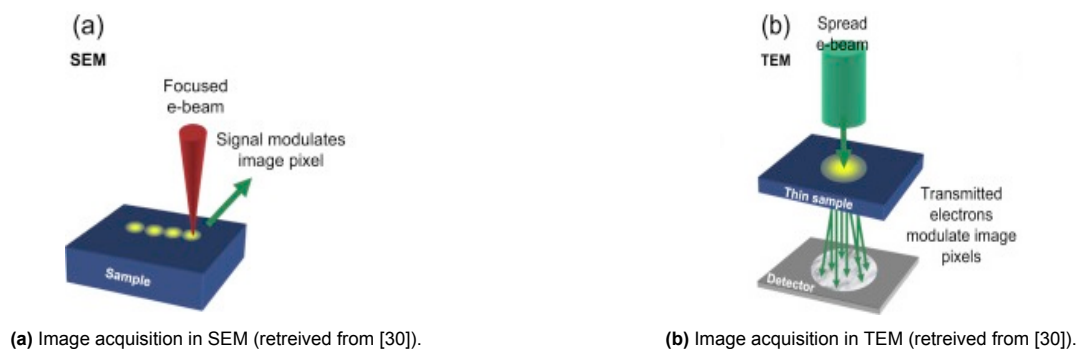
Figure 2.3: Image acquisition in Electron Microscopy methods.
