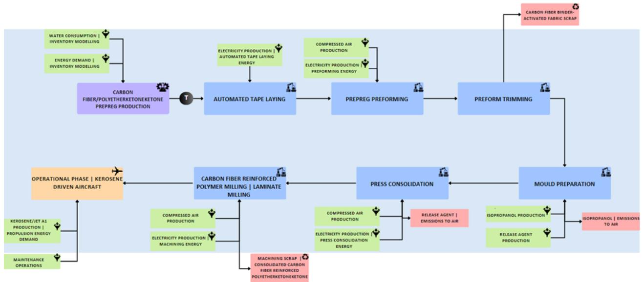
**Figure 7.5:** Process flow of the modelled press consolidated carbon fiber reinforced PEKK product life cycle
