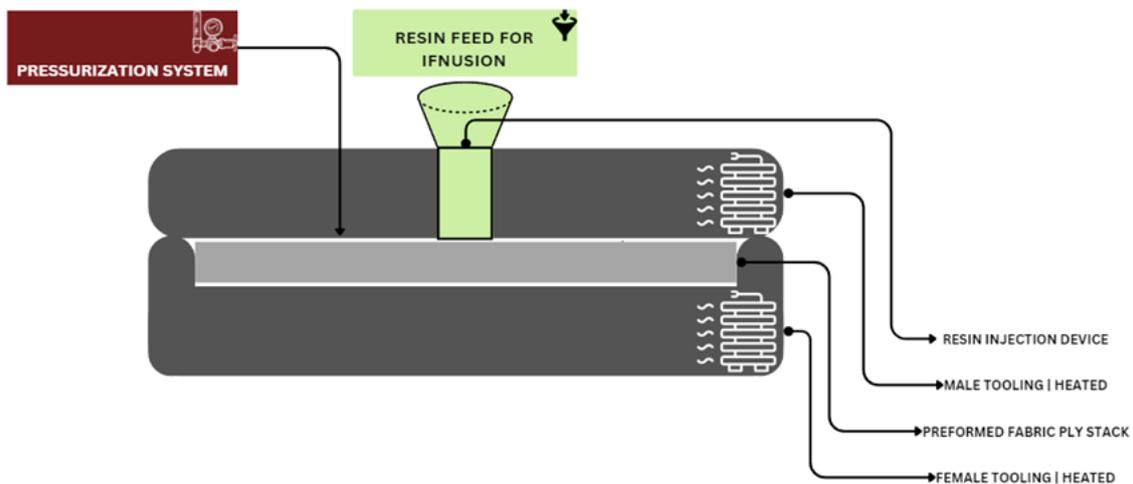
**Figure 7.8:** Simplified illustration of a resin transfer molding cycle
