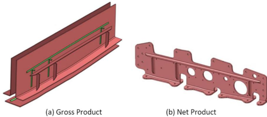
**Figure 6.1:** Illustration of the case study component - wing rib [17] (a) Gross product - precursor to laminate trimming (b) Net product - product at gate [17]
