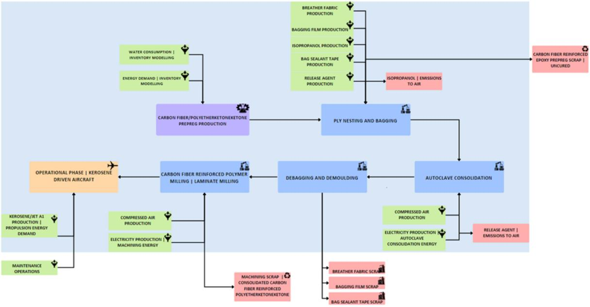
Figure 7.4: Process flow of the modelled autoclave consolidated carbon fiber reinforced PEKK product life cycle
