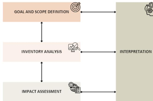
**Figure 5.1:** Stages of a life cycle assessment study based on ISO 1404X:2006 [33]
