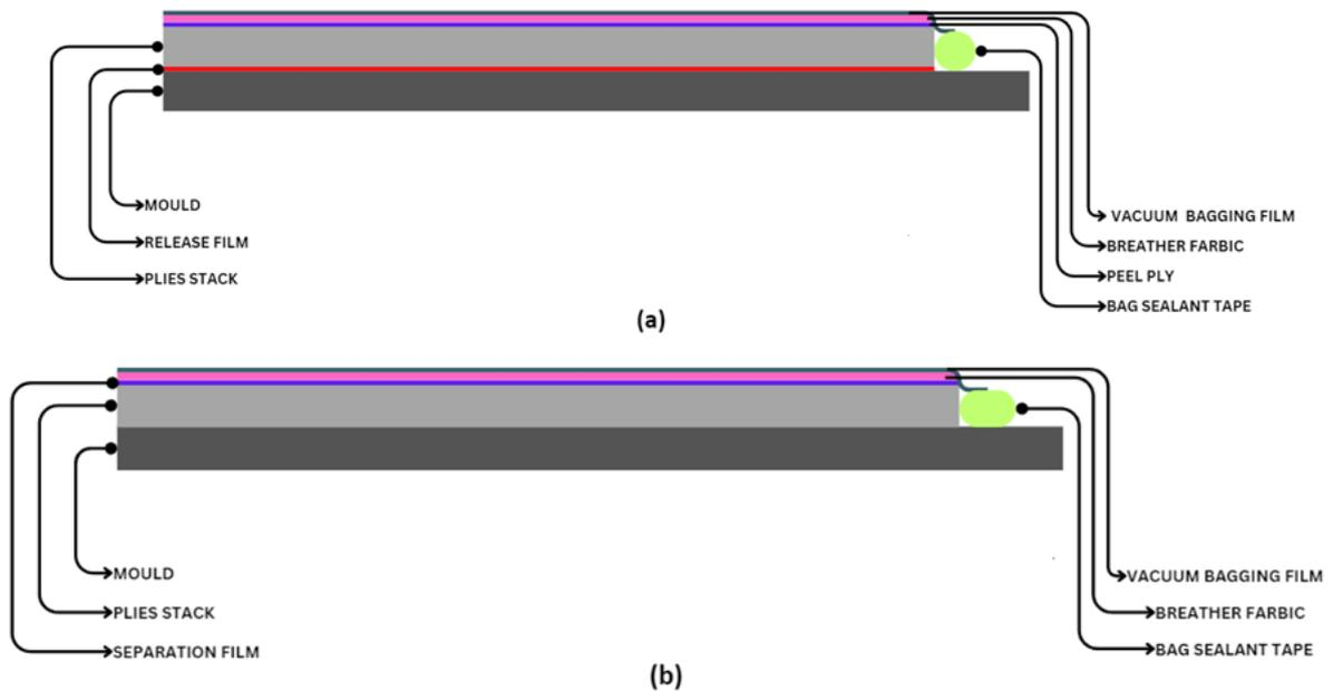
**Figure 7.7:** Simplified illustrations of the buildup over the course of laminate preparation for (a) fiber reinforced thermoset composites, and (b) fiber reinforced thermoplastic composites
