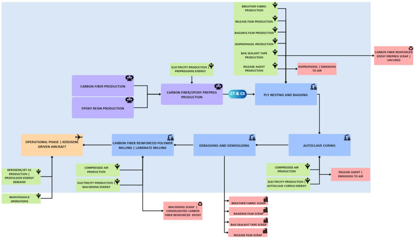
Figure 7.2: Process flow of the modelled autoclave cured carbon fiber reinforced epoxy product life cycle
