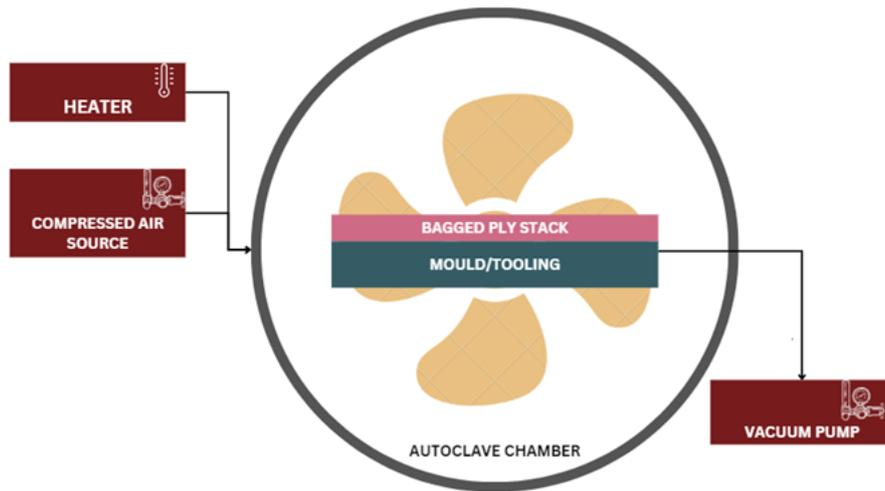
**Figure 7.6:** Simplified illustration of an autoclave cycle constituting a bagged laminate and tooling in the chamber
