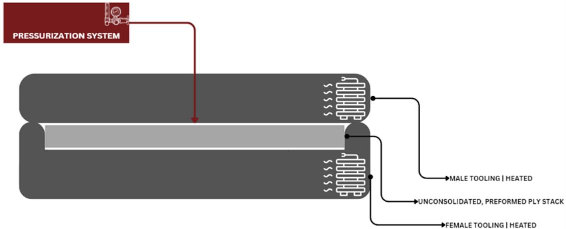
**Figure 7.9:** Simplified illustration of a press consolidation cycle
