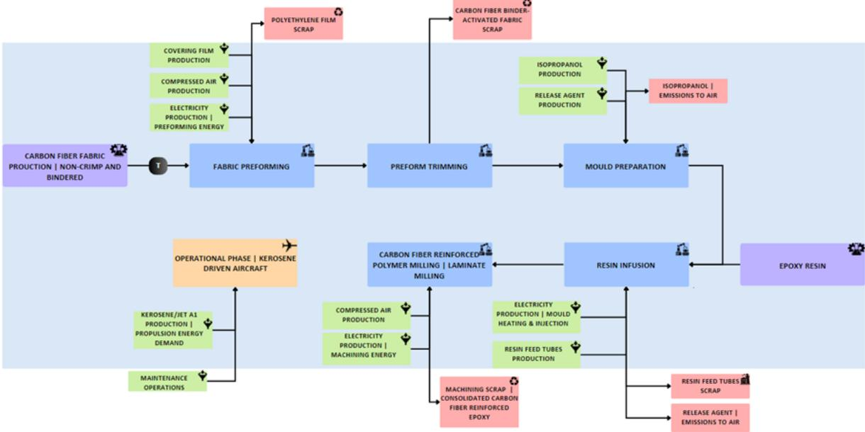
Figure 7.3: Process flow of the modelled resin transfer molded carbon fiber reinforced epoxy product life cycle
