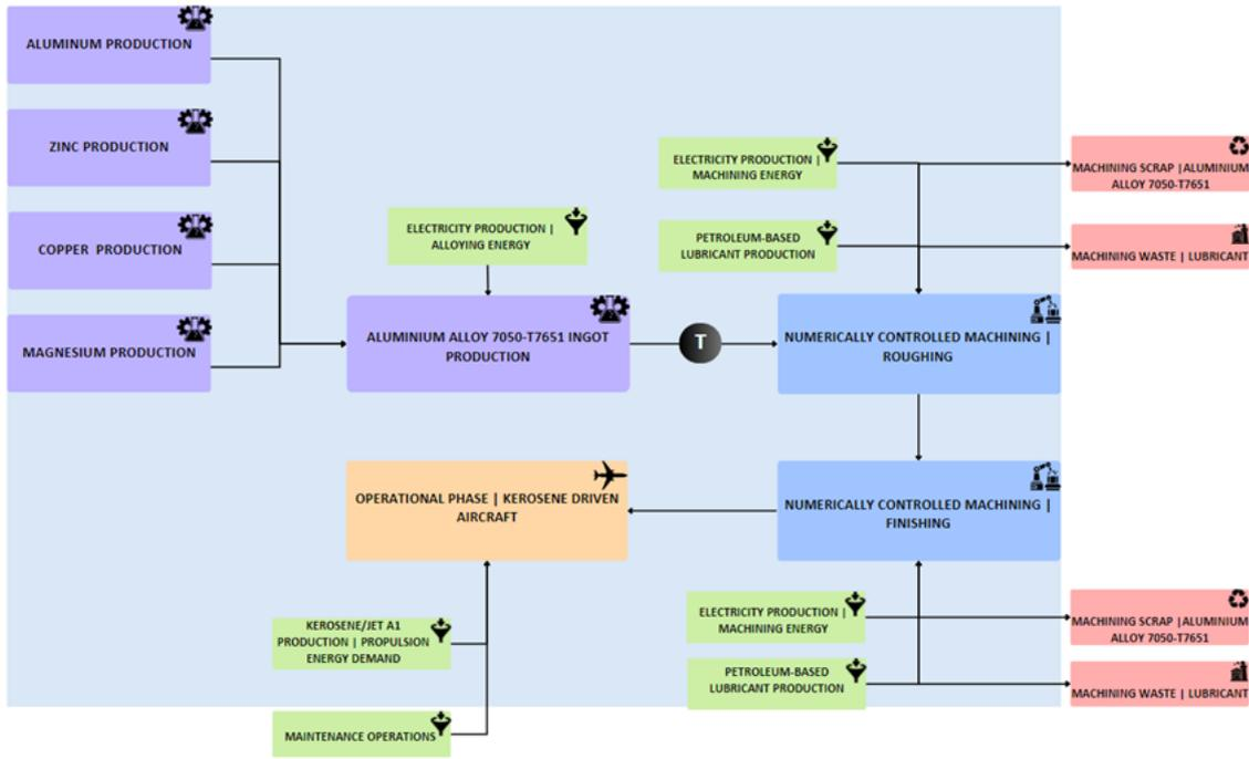
Figure 7.1: Process flow of the modelled numerically machined aluminium alloy 7050-T7651 product life cycle
