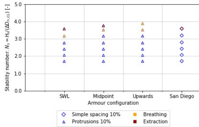
Figure 5.12: Influence of the location of the orientation change on Coastalock stability with 10% protrusions, in the 'PO' configuration with an orientation change at 'SWL' or 'Midpoint', in the 'Upwards' configuration, compared to 10% spacing in the 'San Diego' configuration, under s_{0p} = 0.04 .
