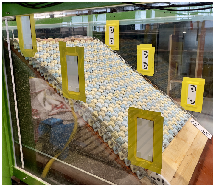
Figure 3.9: SfM test set-up showcasing the GCP pair placement on the flume walls and on the 'Deep Water' foreshore.
