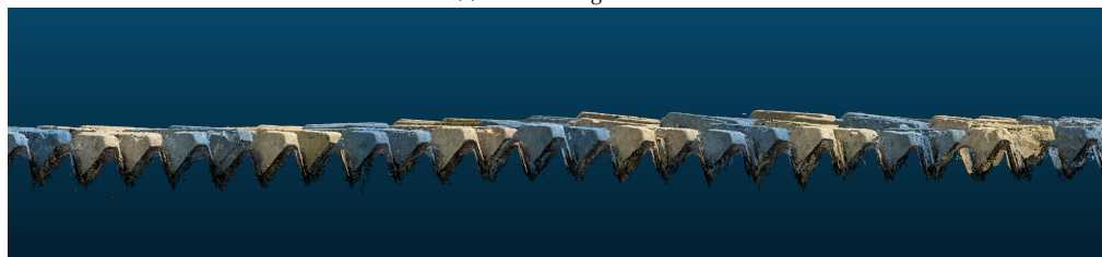
(b) After test run where 'breathing' was first observed, showcasing gradual lifting of several units from the slope.
