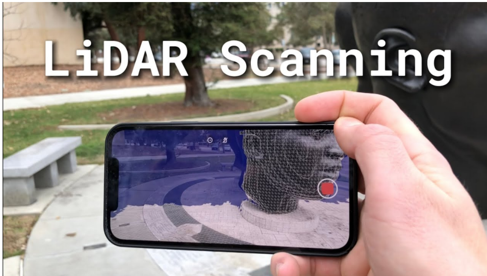
Figure 4: iPhone 12 Pro LiDAR scan Source: Polycam Channel in Youtube
